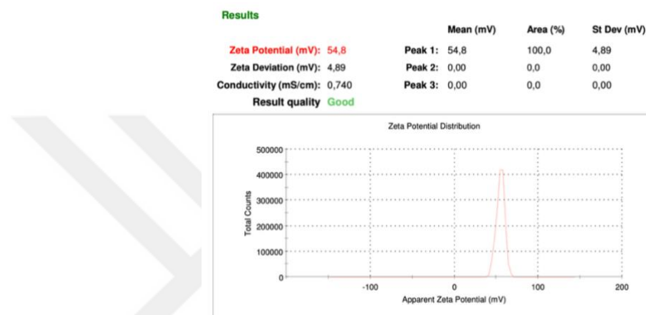
Figure 3.22 Zeta-Potential result of Chi- \text{Fe}_3\text{O}_4 nanoparticles
