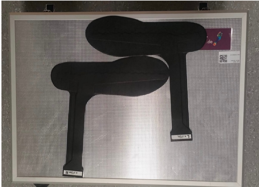
Figure 3. Pedar-X pressure-measuring insoles used for capturing dynamic pressure data during various tasks to record the CoP and vertical forces.
