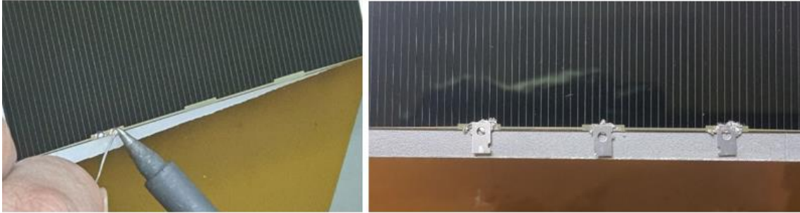
Figure 3.4 : Last try coupons with conventional soldering method.
