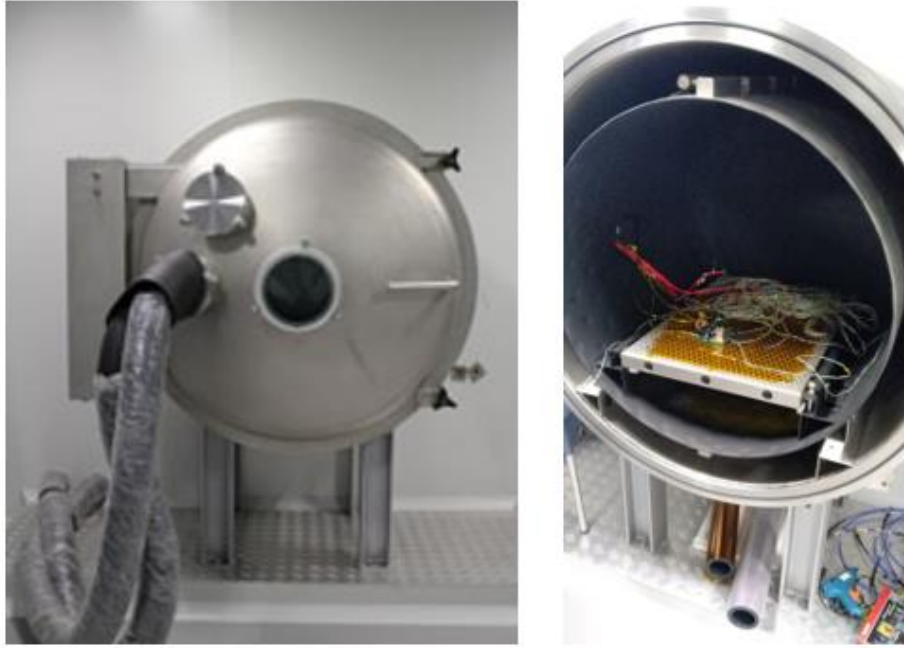
Figure 2.3 : TVAC unit located in the ITU-SDTL laboratory.
