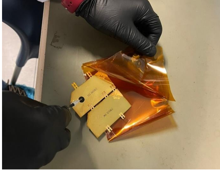
Figure 3.6 : Test coupons developed at TUBITAK MAM.
