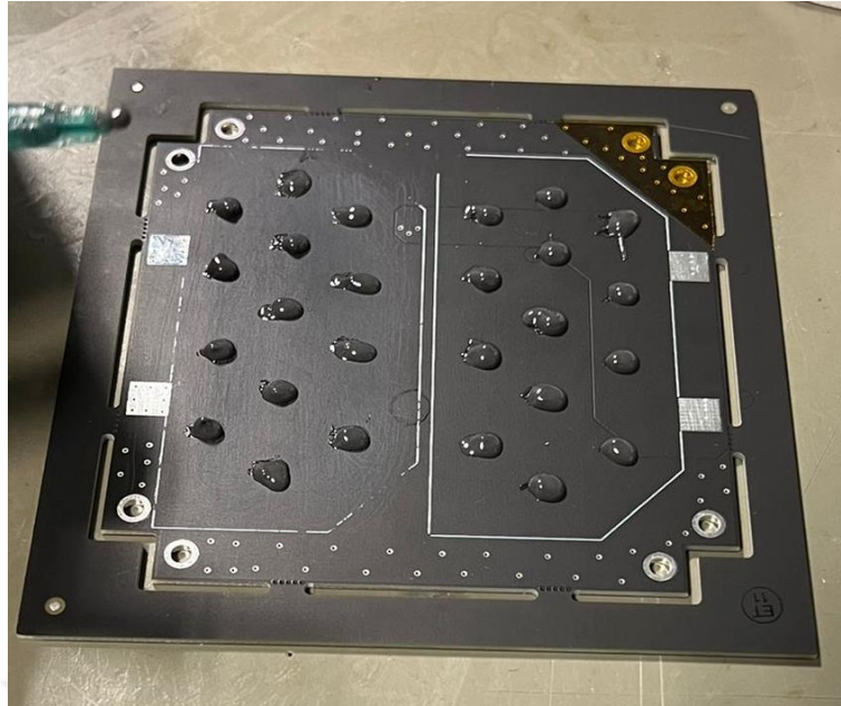
Figure 3.8 : A view of adhesive application for mounting coupon to solar panel.
