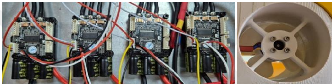
Figure 3.4 : Thruster motor drivers (left). Thruster motors are mounted on the propeller hub (right).
