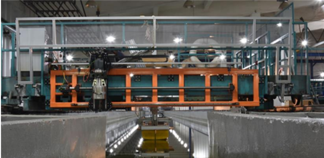
Figure 4.1 : Photograph of the towing vehicle at ITU Ata Nutku Ship Model Laboratory during experimental tests.
