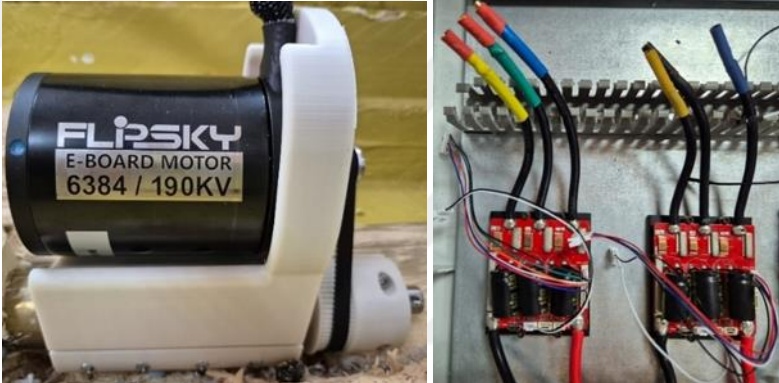
Figure 3.3 : Flipsky motor (left) and VESC 6.9 motor driver (right). Hall effect sensor is located inside the motor.
