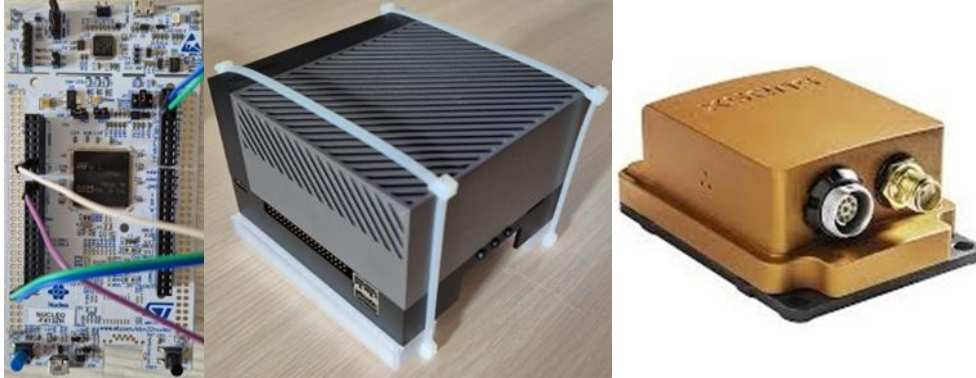
Figure 3.6 : Images of the STM microcontroller (left), ORIN computer (center) and Xsens GPS-IMU (right).
