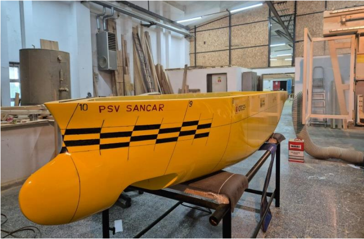
Figure 2.1 : View of the completed PSV Sancar model.
