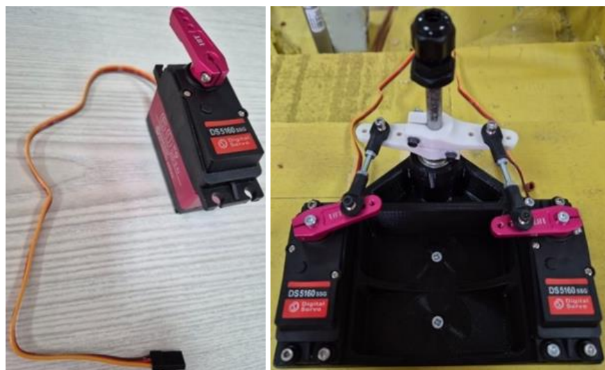
Figure 3.5 : Servo motor (left). Dual servo motor assembly for the starboard rudder of the vessel (right).
