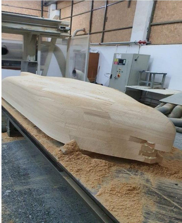
Figure 2.3 : CNC-machined wooden ship hull model.
