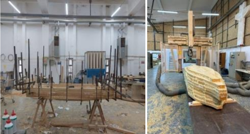
Figure 2.2 : Rough model fabrication of the PSV hull.
