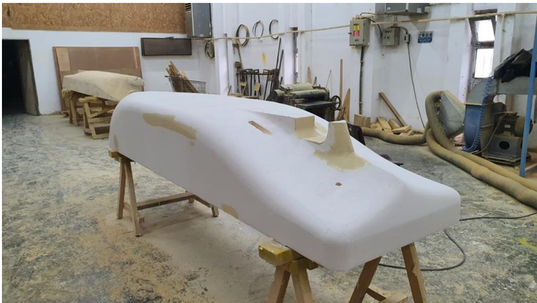
Figure 2.4 : Finished PSV hull after CNC and priming.
