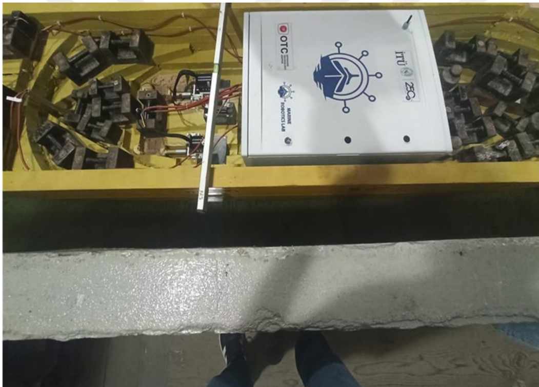
Figure 4.2 : Layout of the electronic control box and lead ballast blocks during the trim-calibration procedure.
