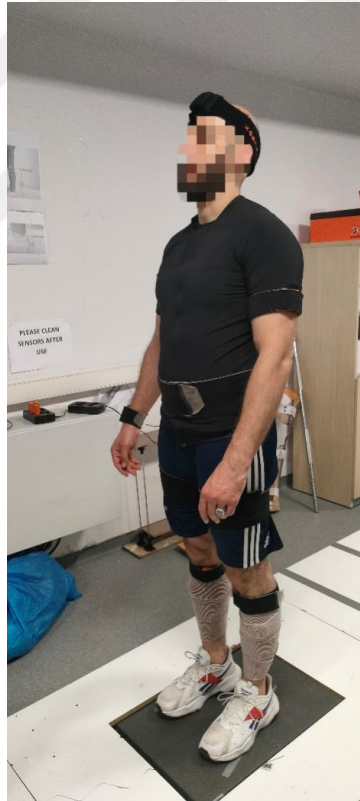
Figure 11. Movella xsens motion capture system sensor placement.
