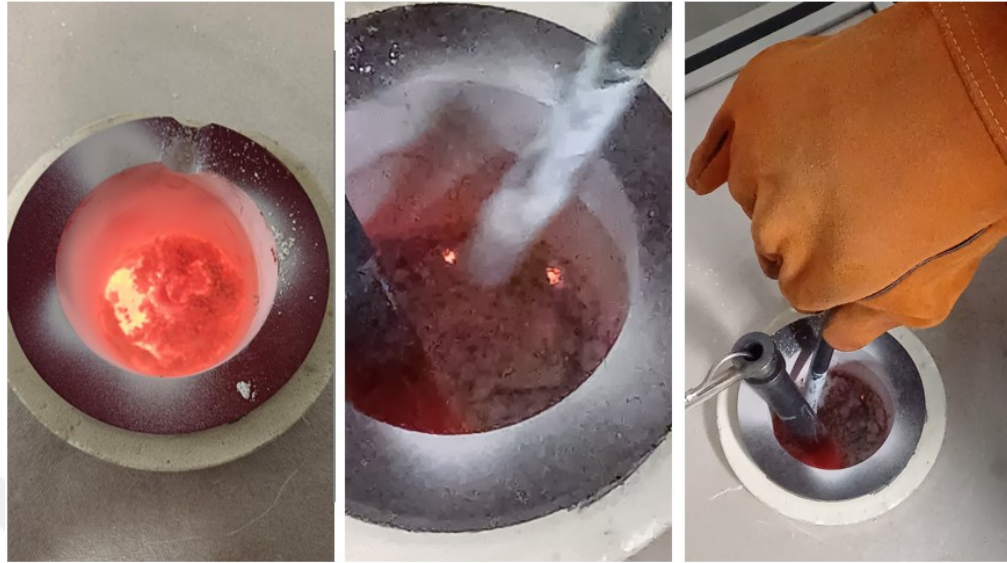
Figure 3.7. Induction furnace production process melting, mixing, and stirring of Al MgO.
