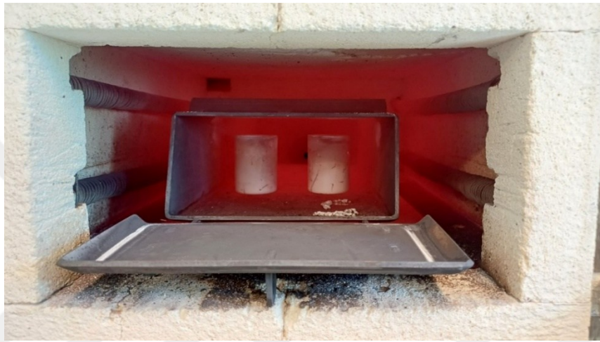
Figure 3.6. Muffle furnace with alumina crucibles containing raw materials.
