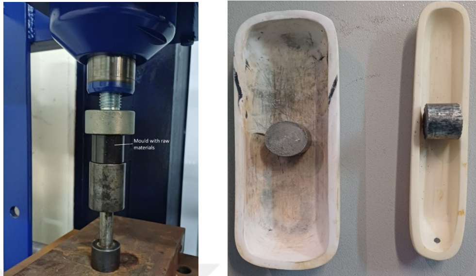
Figure 3.8. Manual compression device with raw materials (left) and Compressed Al-MgO powder into coins in boat crucibles.
