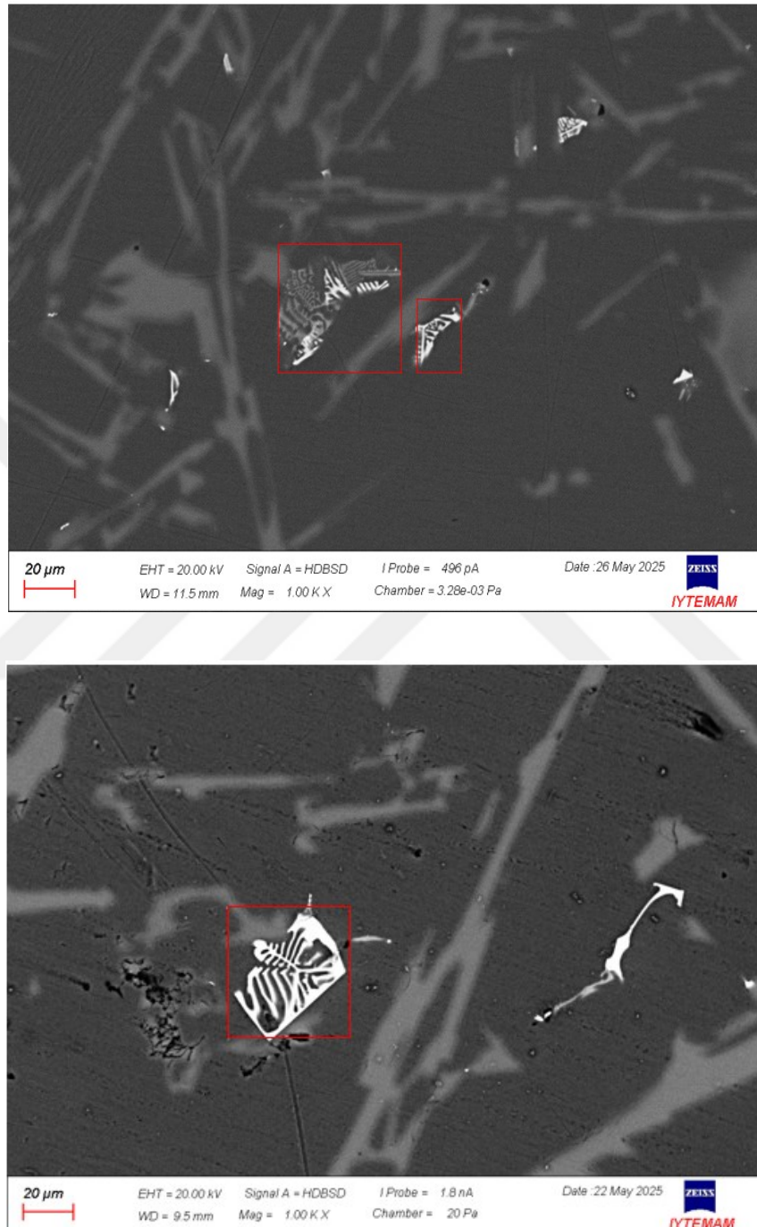
Figure 4.10. SEM image of experiment 10 & 4 showing script like phase in matrix formed due to high Fe content (red box)).
