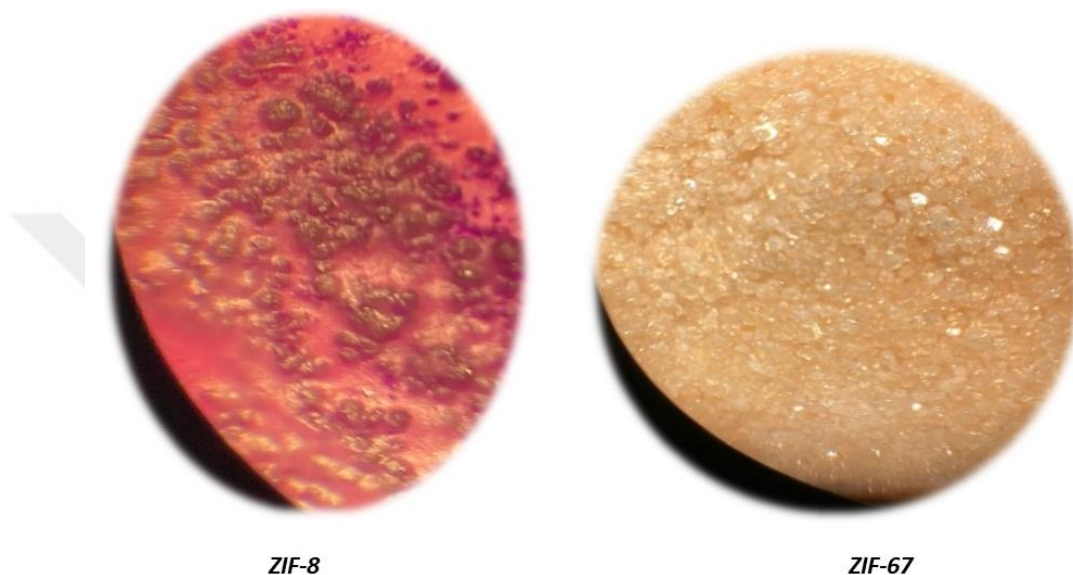
Figure 3.4: Optical Micrographs of ZIF-8 and ZIF-67 Crystal Morphologies
