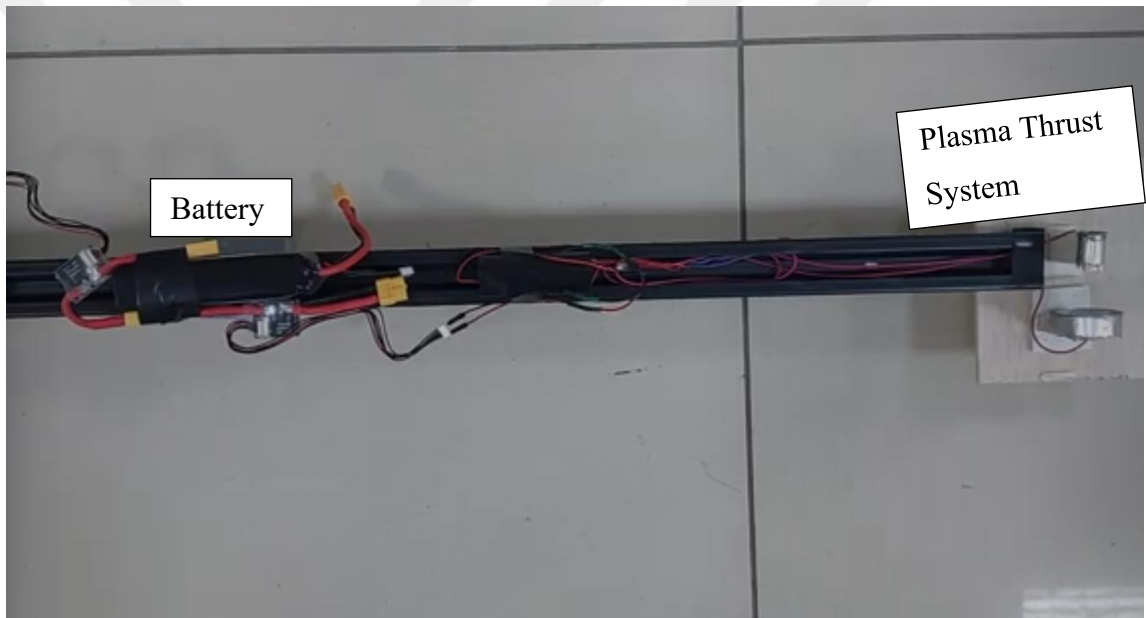
Figure 3.9 Sample battery-powered speed measurement system (Experiment Setup2)
