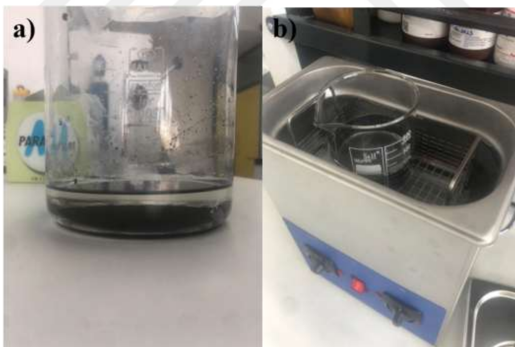
Figure 9. Graphite oxide that settles to the bottom because of resting (a) The ultrasonic bathing phase of graphite oxide (b)
