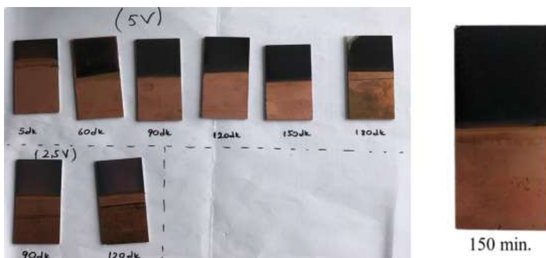
Figure 12. The plates were covered with the EPD process and the best-coated plate image at 5V for 150 minutes
