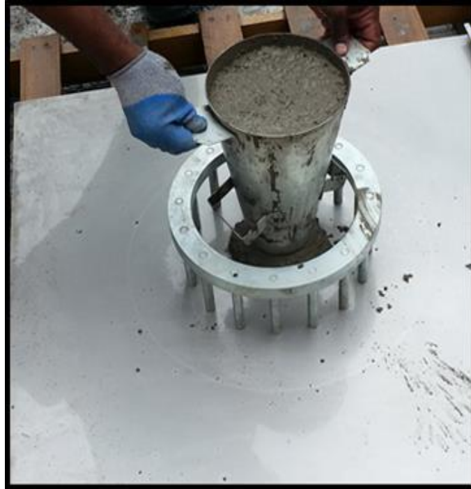
Figure 2.15 J-ring test (Hadiwidodo and Mohd, 2008)
