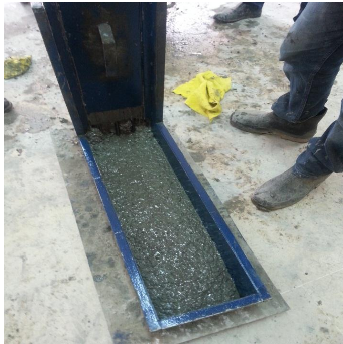
Figure 3.5 Photographic view of L-box apparatus and testing procedure
