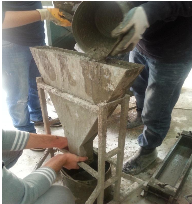
Figure 3.4 Photographic view of V-funnel flow time measurement
