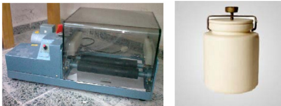
Figure 7. Pascall Engineering, 1600-VS-A roll mixer) and alumina jar
