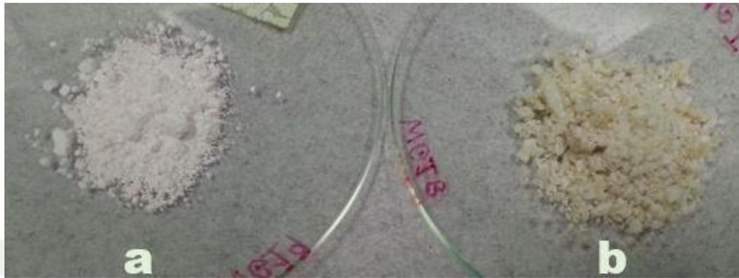
Figure 6.19 Image of (a) pure  $\text{MgCl}_2$  and (b) reacted particles (with an expected chemical structure of  $\text{MgCl}_2 \cdot n\text{H}_2\text{O} \cdot m\text{HCl}$ )
