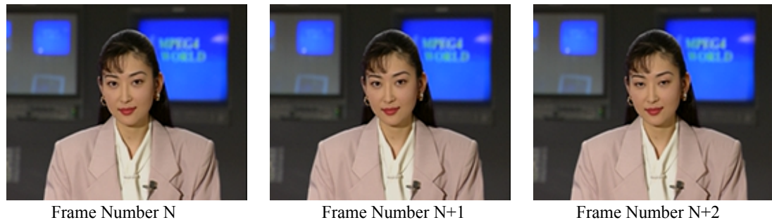
Figure 2 Illustration of temporal redundancy in a video signal
