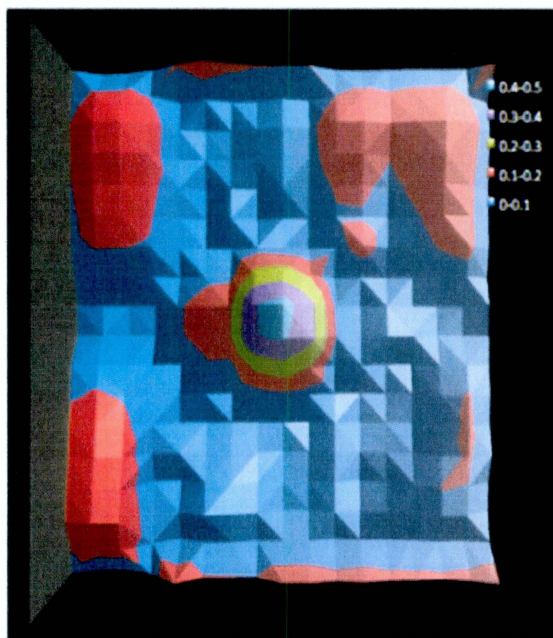
Figure 3.10: The 3-D plot of the non-uniformity deviation of the PMT (S.N: JA0883)
