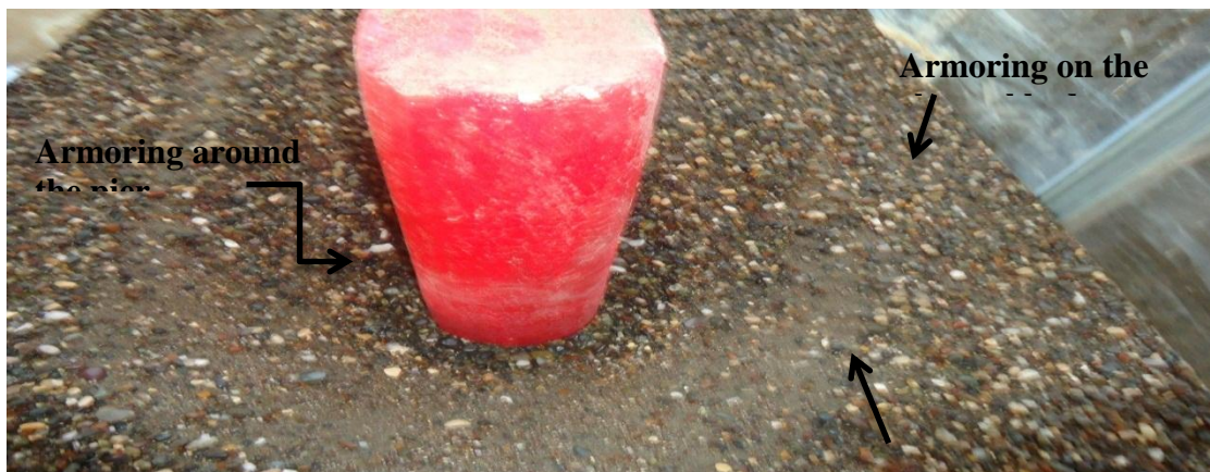
Figure 4.7 Armoring the channel bed and in the scour hole
