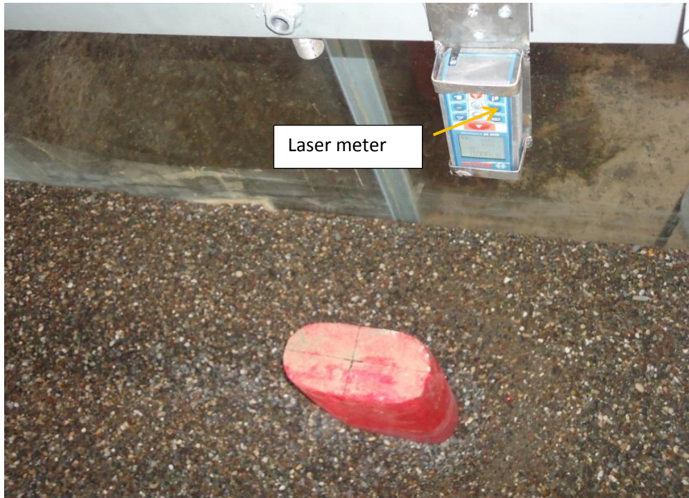
Figure 3.3 Laser meter installed in the channel
