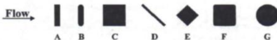
Figure 2.7 the shapes A to G on the scour depth relative to a circular pier (Melville, 2000)
