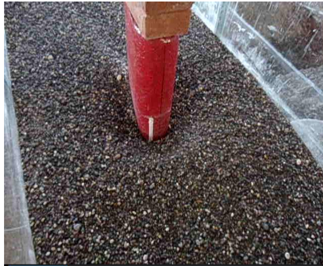
Figure 4.2 Scoured bed around A1, A2 and A5, Q= 58 \text{ l/s}
