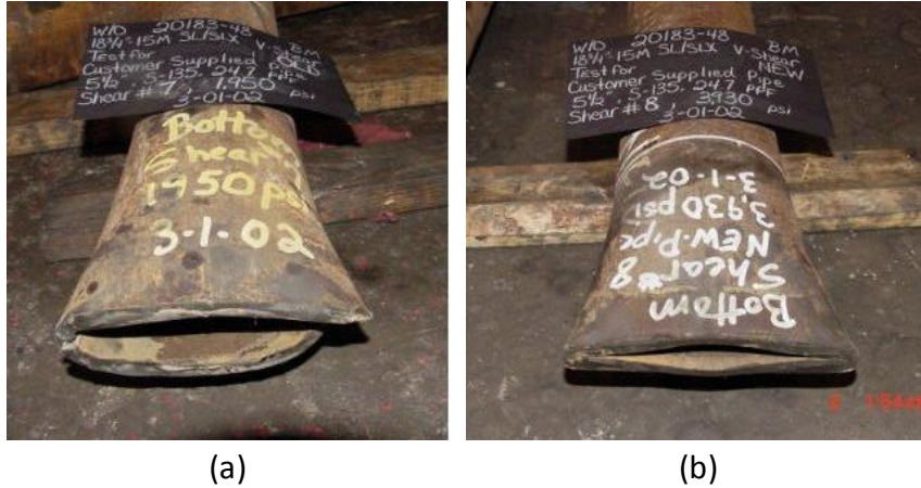
Figure 11 Two sheared tubes with same material grade and cross sectional area: (a) Required 1,950 psi to shear, (b) Required 3,930 psi [Childs et. al., 2004]
