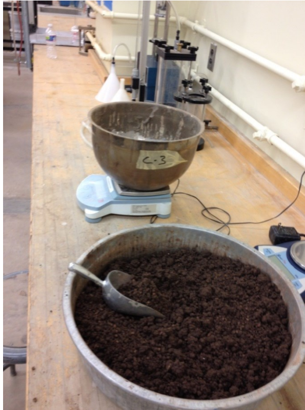
Figure A18. Preparing for Weighing Soil Samples before Compaction.
