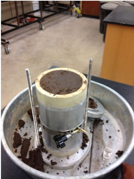
Figure A25. Preparing to Take It Out after Fourth Layer Compaction.
