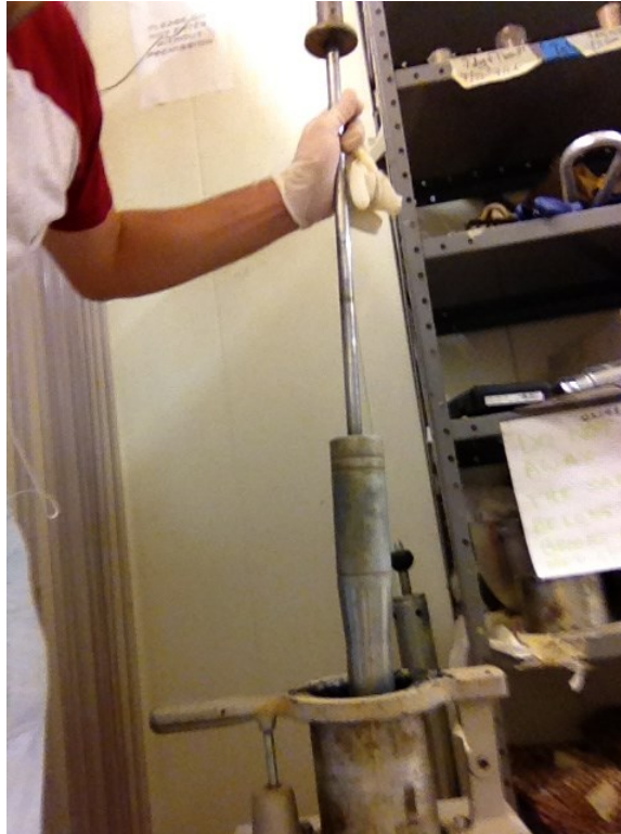
Figure A2. Plastic Asphalt Compactor.
