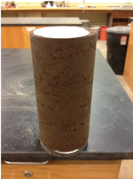
Figure A31. After MTS Test, Taking Weight and Height and Moisture Content.
