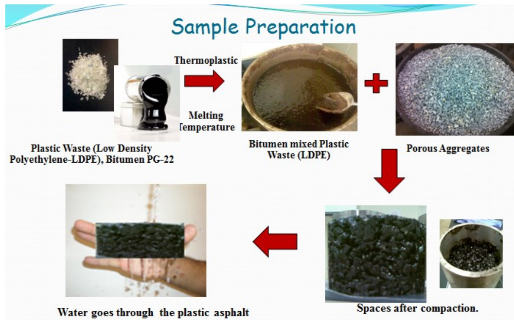
Figure A1. Sample Preparations for Permeable Plastic Asphalt that Mixing of LDPE, Porous Aggregates, and Binder to Create.
