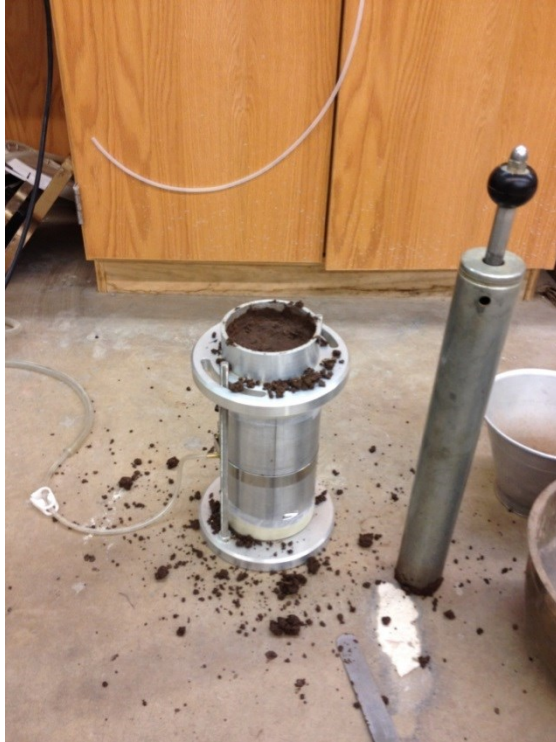
Figure A24. After the Fourth Layer Compaction.
