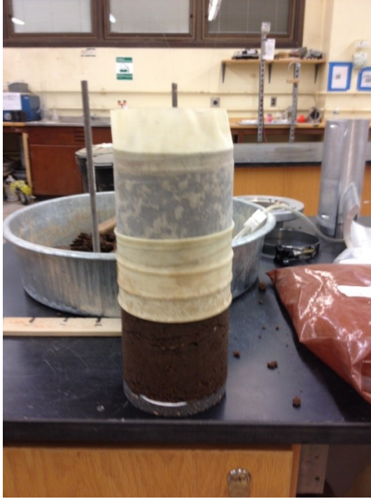
Figure A26. Covering with Membrane to Obtain Height and Weight before MTS Test.
