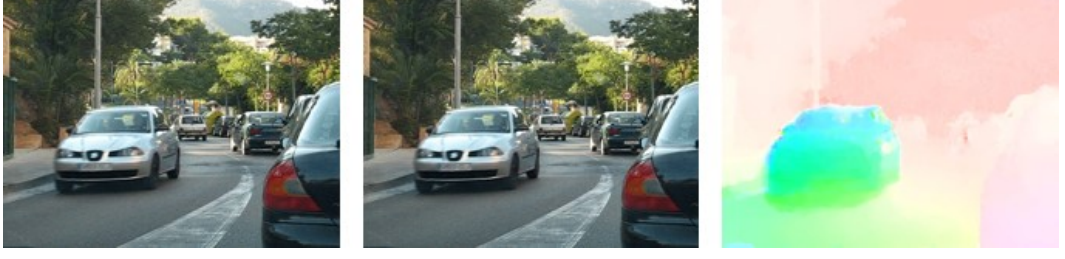
Figure 2.5. The optical flow map shown in the third column is computed between the first and the second image. It is created by tracking the points between two consecutive frames in both x and y direction, and combining them into a single map.
