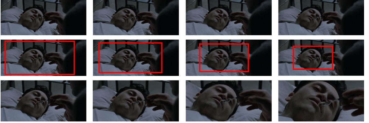
Figure 2.7. An example zoom-in effect. The rows are: original frames, crop window, retargeted frames successively. Although in the camera is still in the original frames, the retargeted frames show a zoom-in effect. The reason is the decreasing crop window size, which is represented with a red box in the second row.
