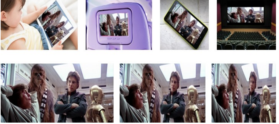
Figure 1.1. The first row illustrates viewing a movie in various sized displays. The second row contains three aspect ratios; 21 : 9, 16 : 9 and 4 : 3 respectively. The original frame is taken from Star Wars: The Empire Strikes Back movie where the actual aspect ratio is 2.35 : 1, which is quite close to the first image. In the third image, the objects are stretched and squeezed, which will decrease the viewing quality.
