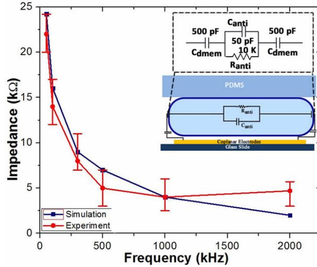
Figure 5.23: Impedance fitting of antibody serum droplet.
