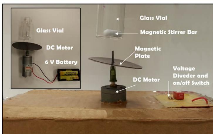
Figure 4.9: Magnetic stirrer and source connections.
