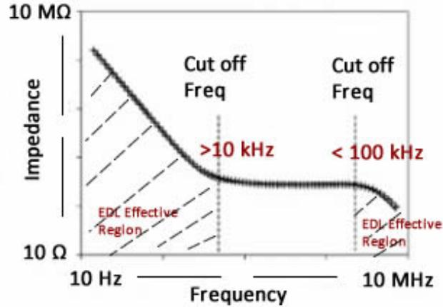
Figure 5.21: Frequency response of analytes impedance in the channel based on the EDL formation.
