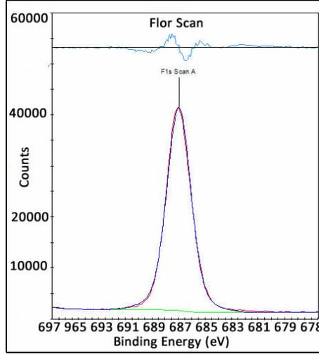
Figure 3.11: XPS measurement result of the PDMS surface that was used in Modification-B, percentage of the Fluor molecule concentration was % 72.
