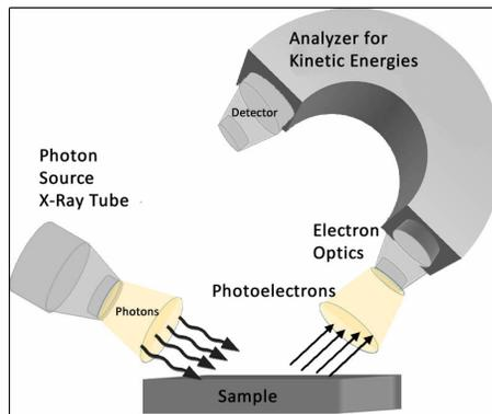
Figure 3.9: Schematic of XPS working mechanism.
