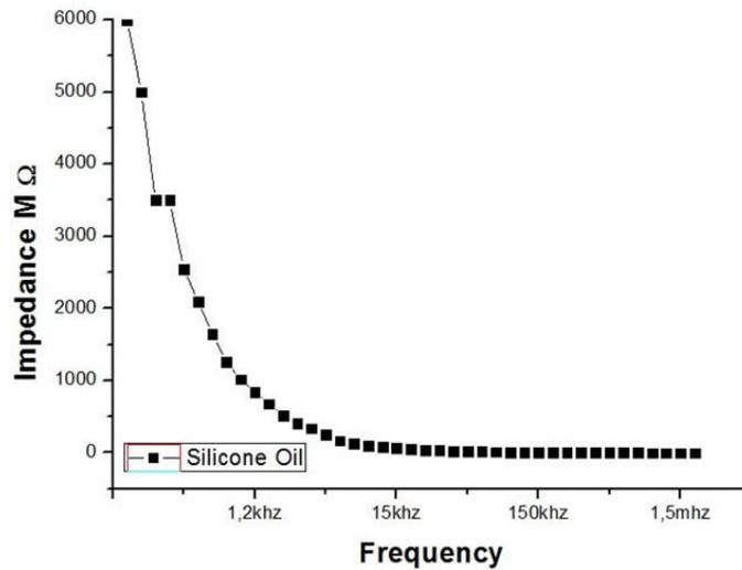
Figure 5.17: Frequency response of silicone oil impedance in microchannel.
