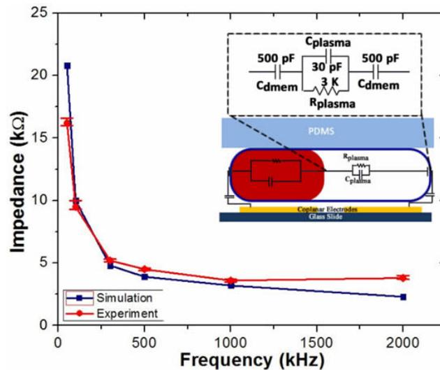
Figure 5.27: Impedance fitting of antibody sera and PBS mixture part of agglutinated blood droplet.
