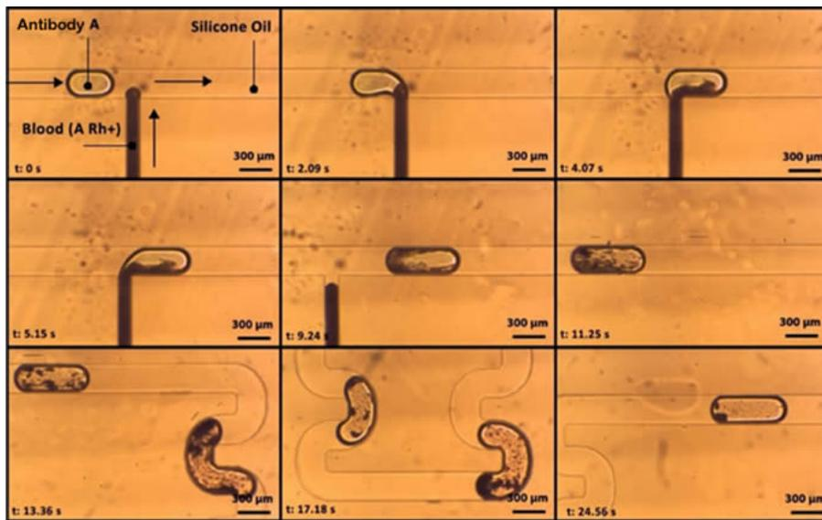
Figure 3.28: Microscope image of droplet formation and blood sample injection in the channel.
