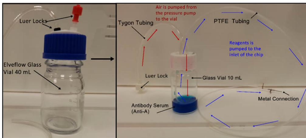
Figure 4.8: Glass vials and fluid flow direction.
