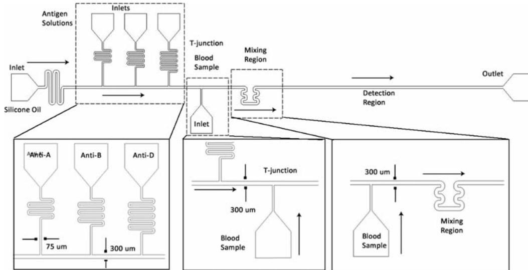
Figure 3.27: Schematic of microfluidic channel design.
