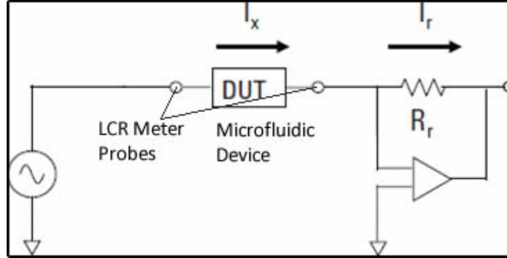
Figure 4.5: Illustration of circuit of LCR Meter connection to DUT.
