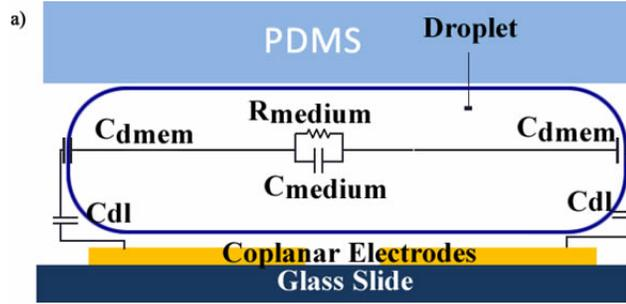
Figure 5.2: Equivalent circuit of microchannel with droplet ( $C_{dmem}$  is droplet membrane,  $R_{medium}$  and  $C_{medium}$  are the resistance and capacitance of the reagent in the droplet, and  $C_{dl}$  is electrical double layer capacitance).
