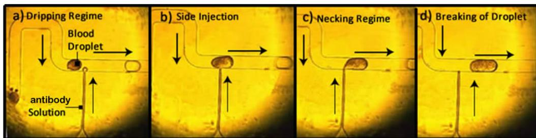
Figure 3.25: Microscope image of droplet formation using silicone oil in flow focusing channel design and injection of antibody serum from the side channel.
