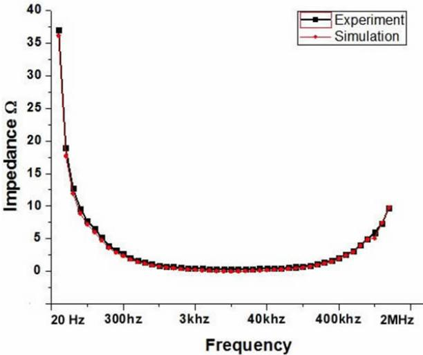
Figure 5.15: Fitting of experimental data with the simulation results for 220  $\mu\text{F}$  capacitor.
