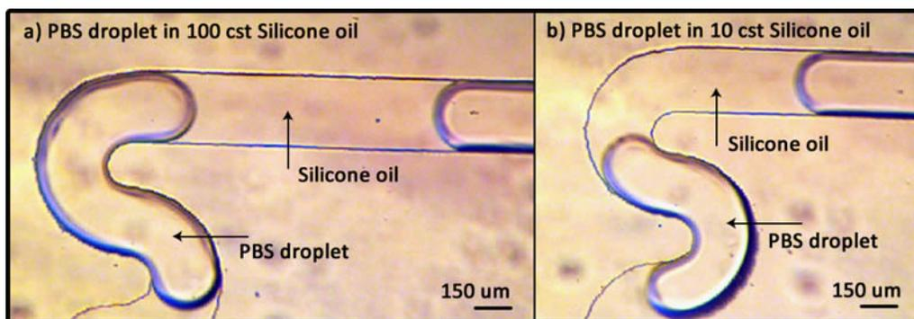
Figure 3.18: Microscope image of PBS droplet formation in T-junction.
