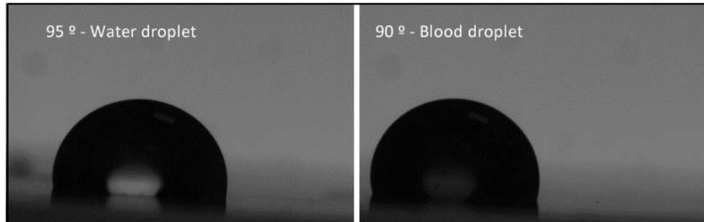
Figure 3.15: Measured contact angle of PDMS that was treated using modification D.
