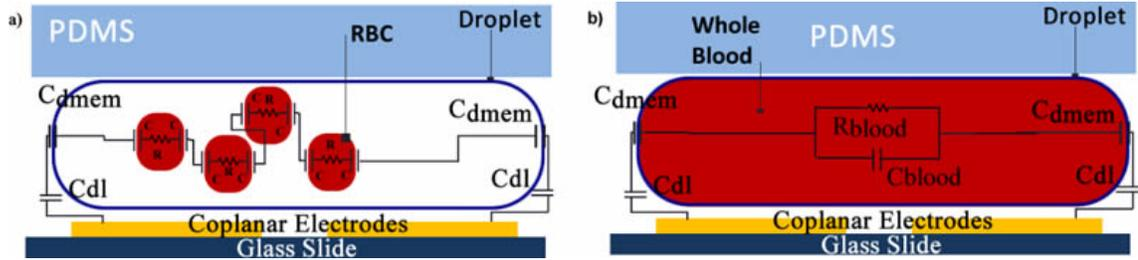
Figure 5.3: Equivalent circuit of microchannel with cells in droplet a) illustration of individual cells in droplet b) illustration of approximation of cells as a homogeneous analyte.
