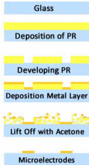
Figure 3.5: Schematic of lift off process.
