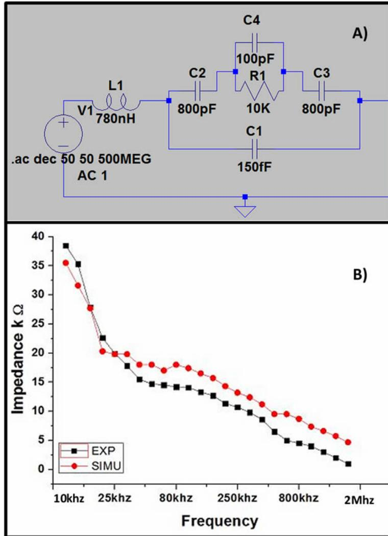
Figure 5.20: Circuit design for antibody sera in the simulation (a) and fitting results (b).
