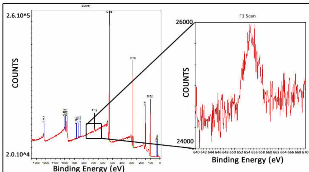
Figure 3.10: XPS measurement result of the PDMS surface that was used in Modification-A, percentage of the Flor molecule concentration was % 1.62.
