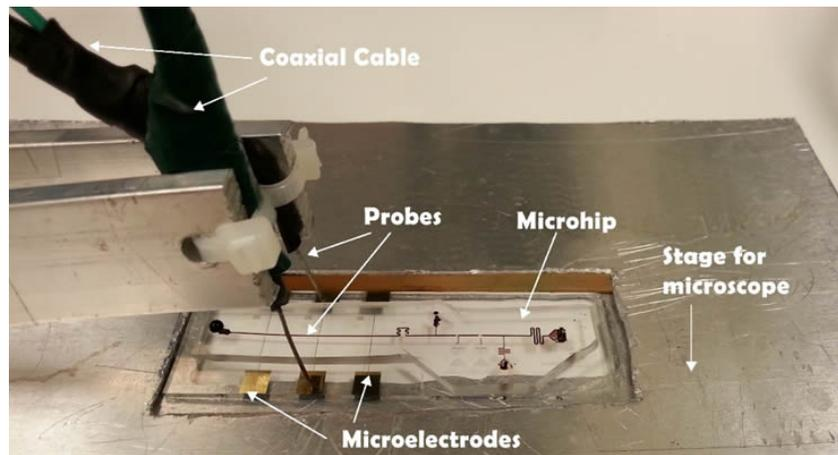
Figure 4.6: Probes of the LCR Meter.
