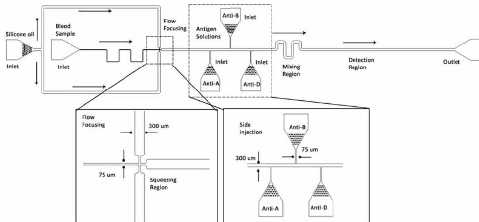
Figure 3.26: Schematic of microfluidic channel design.
