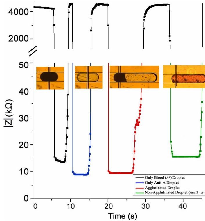
Figure 4.10: Impedance of four different droplets in the combination a) impedance of whole blood droplet -  $13\text{ k}\Omega$  b) droplet of antibody solution -  $9\text{ k}\Omega$  c) agglutinated droplet clusters - ( $30\text{-}34\text{ k}\Omega$ ), mixture antibody-PBS - ( $10\text{ k}\Omega$ ) d) non-agglutinated droplet -  $15\text{ k}\Omega$ .
