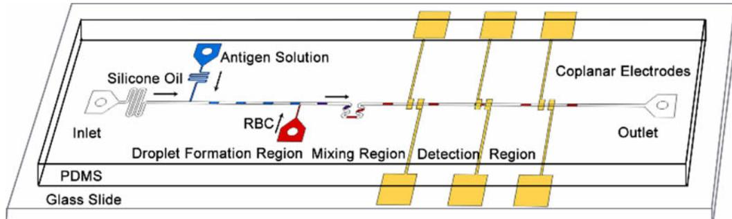
Figure 4.2: Schematic of final microchannel design.
