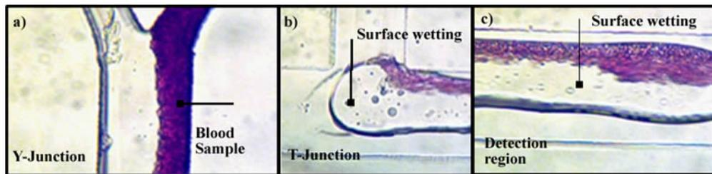
Figure 3.17: Microscope image of PDMS surface wetting.
