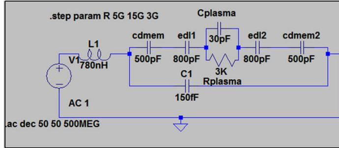
Figure 5.26: Circuit design for antibody sera and PBS mixture part in the simulation.
