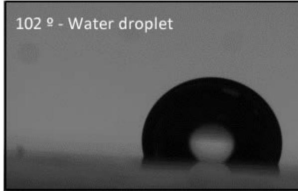
Figure 3.14: Measured contact angle of PDMS that was treated using modification C.
