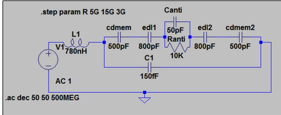
Figure 5.22: Circuit design for antibody sera droplet in the simulation.
