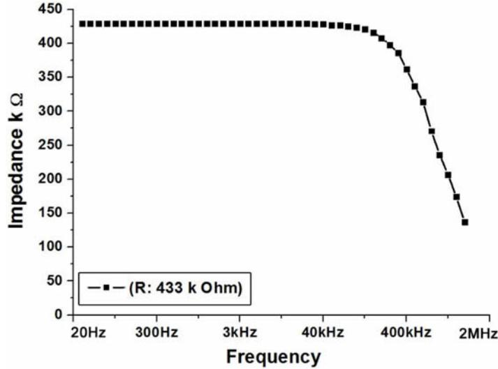
Figure 5.6: Frequency response of impedance for 433 k $\Omega$ .
