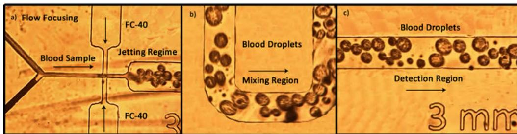
Figure 3.21: Microscope image of droplet formation in jetting regime.
