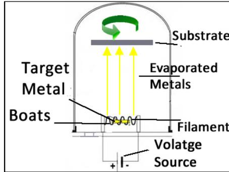
Figure 3.4: Schematic of deposition in thermal evaporator system.
