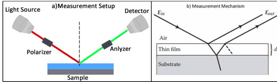
Figure 3.7: Schematic of ellipsometer measurement setup (a) and measurement method (b).
