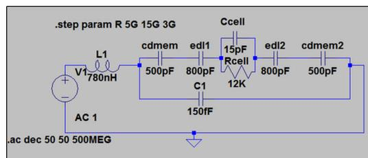
Figure 5.24: Circuit design for whole blood droplet in the simulation.
