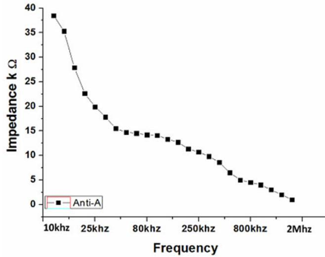
Figure 5.19: Frequency response of antibody sera impedance in microchannel.
