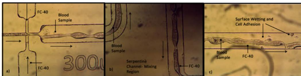
Figure 3.22: Microscope image of surface wetting (a) flow focusing region, (b) serpentine part of the channel, (c) detection region of the channel.
