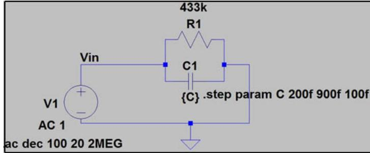
Figure 5.8: Circuit design in the simulation to determine stray capacitance.
