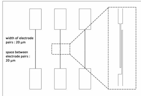
Figure 3.29: Schematic of microelectrode design.
