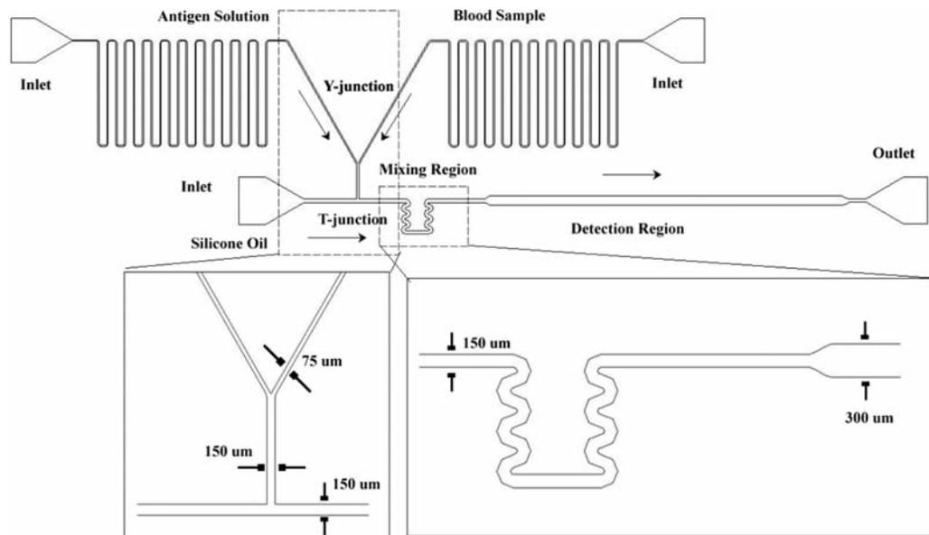
Figure 3.16: Schematic of microfluidic channel design.
