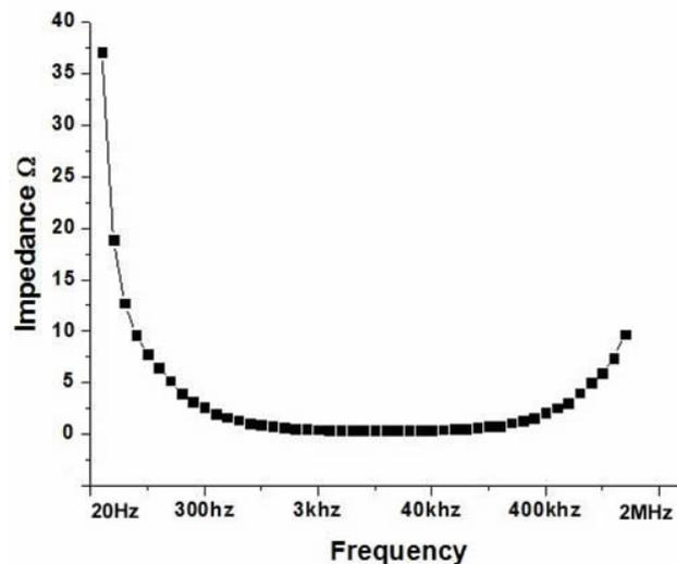
Figure 5.12: Frequency response of impedance for 220  $\mu\text{F}$ .
