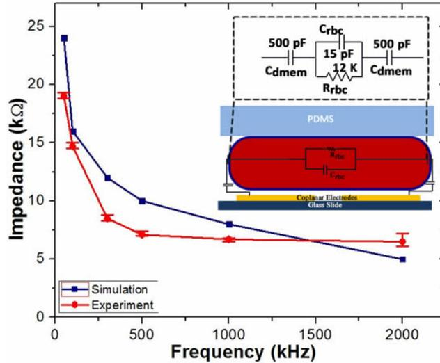
Figure 5.25: Impedance fitting of whole blood droplet.
