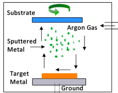
Figure 3.3: Schematic of deposition in sputtering system.
