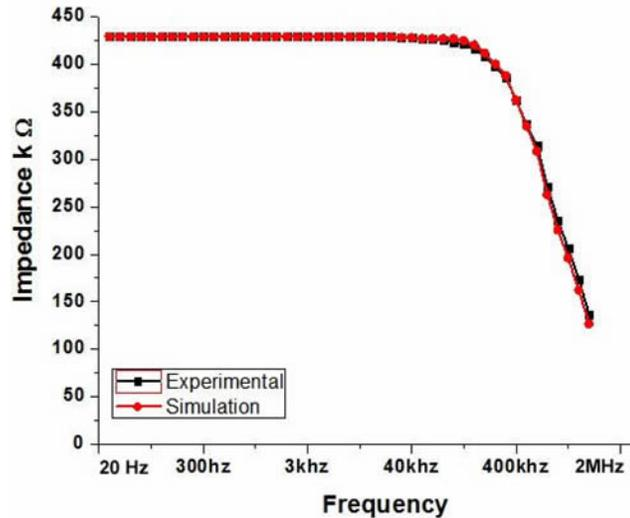
Figure 5.10: Fitting of experimental data with the simulation results for 433 kΩ resistor.
