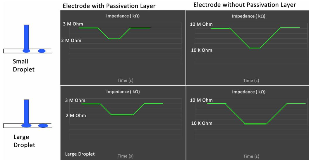
Figure 3.30: Illustration of data acquisition with passivated and bare electrodes.
