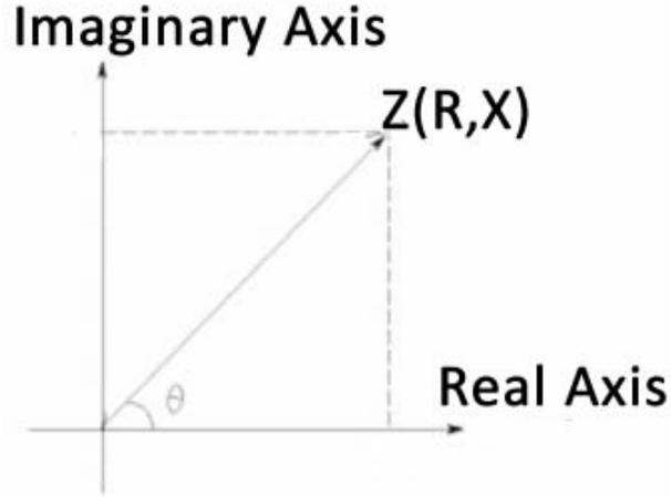
Figure 4.1: Illustration of impedance in coordinate system.
