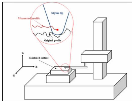
Figure 3.8: Schematic of a profilometer and measurement method.
