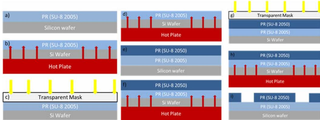
Figure 3.1: Schematic of photolithography process for SU-8 2050.
