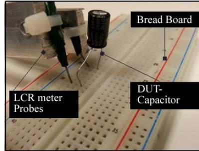
Figure 5.11: Image of capacitor connection to probes.
