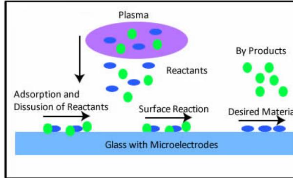
Figure 3.6: Schematic of reaction mechanism in PECVD.
