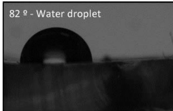
Figure 3.13: Measured contact angle of PDMS that was treated using modification B.
