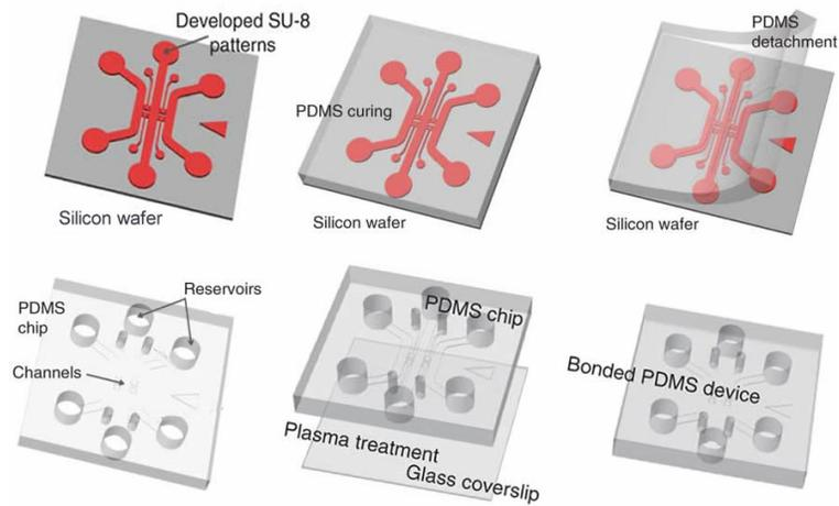
Figure 3.2: Schematic of softlithography process for PDMS microchannel.
