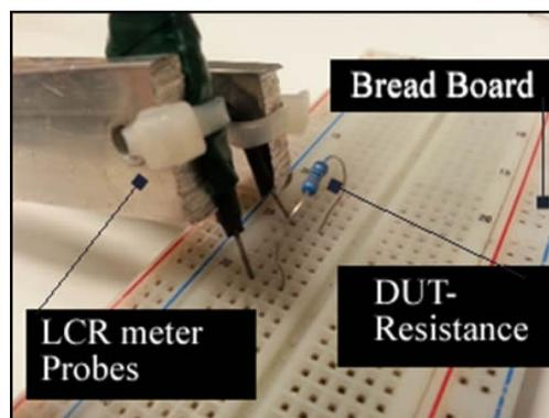
Figure 5.5: Image of resistor connection to probes.
