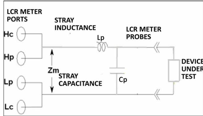
Figure 5.16: Schematic of final circuit design of LCR Meter.
