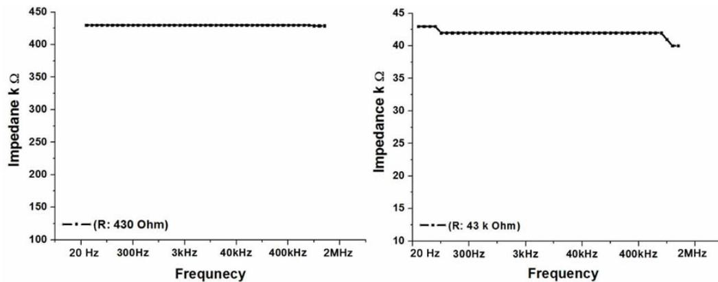
Figure 5.7: Frequency response of impedance for 43 kΩ (a) and 433 Ω (b).
