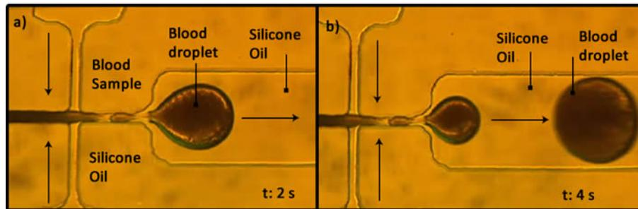
Figure 3.24: Microscope image of droplet formation using silicone oil in flow focusing channel design.
