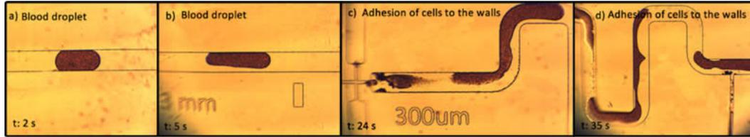
Figure 3.23: Microscope image of droplet formation in fluorinated channel (a) single droplet in flow focusing region, (b) droplet that was flowing through the outlet, (c,d) sticking of the blood sample to the surface.
