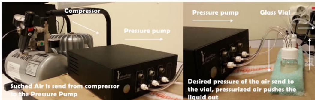
Figure 4.7: Pressure pump and vial connection.
