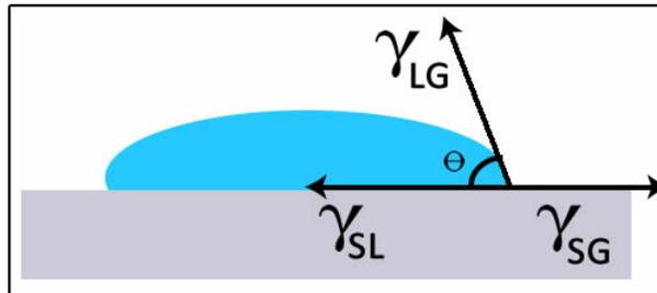
Figure 3.12: Illustration of contact angle and surface tension between surfaces.
