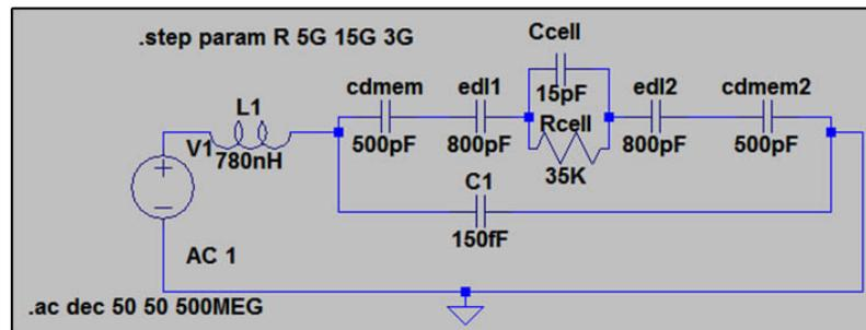
Figure 5.28: Circuit design for cluster part of agglutinated droplet in the simulation.
