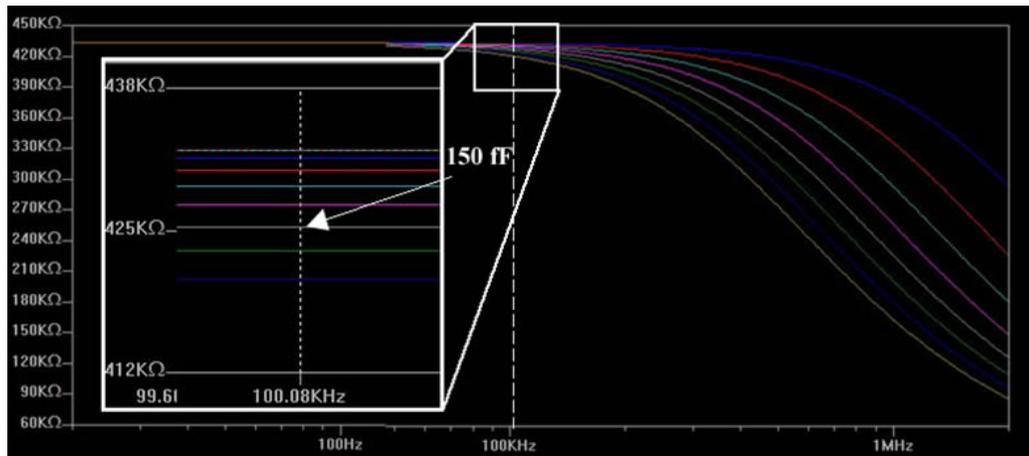
Figure 5.9: Simulation result for stray capacitance.
