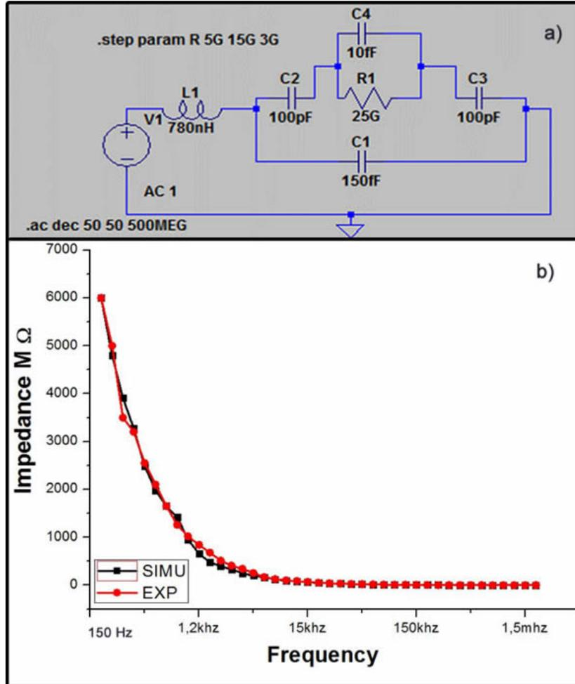
Figure 5.18: Circuit design for silicone oil in the simulation (a) and fitting results (b).
