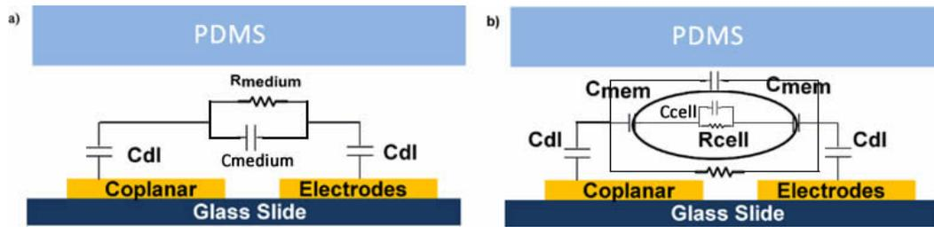
Figure 5.1: Equivalent circuit model of microchannel a) channel without cell,  $C_{dl}$  is electrical double layer,  $C_{medium}$  is the capacitance of of the medium,  $R_{medium}$  is the resistance of the medium b) channel with cell,  $C_{dl}$  electrical double layer,  $C_{cell}$  and  $R_{cell}$  are the capacitance and the resistance of the cells and  $C_{mem}$  is the membrane capacitance of the cell.
