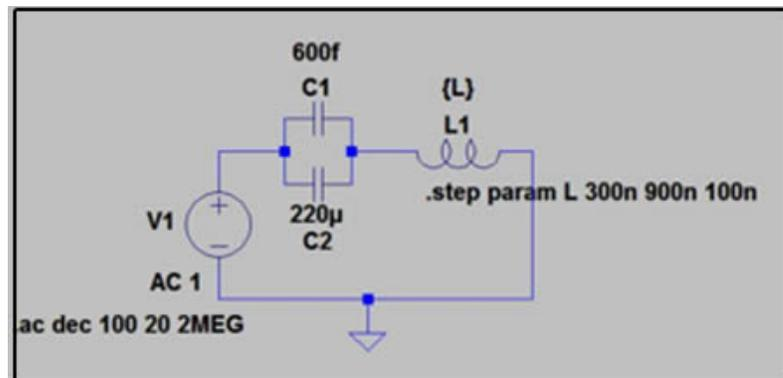
Figure 5.13: Circuit design in the simulation to determine stray inductance.
