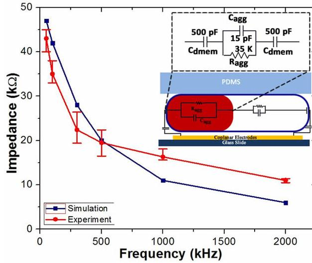
Figure 5.29: Impedance fitting of cluster part of agglutinated blood droplet.
