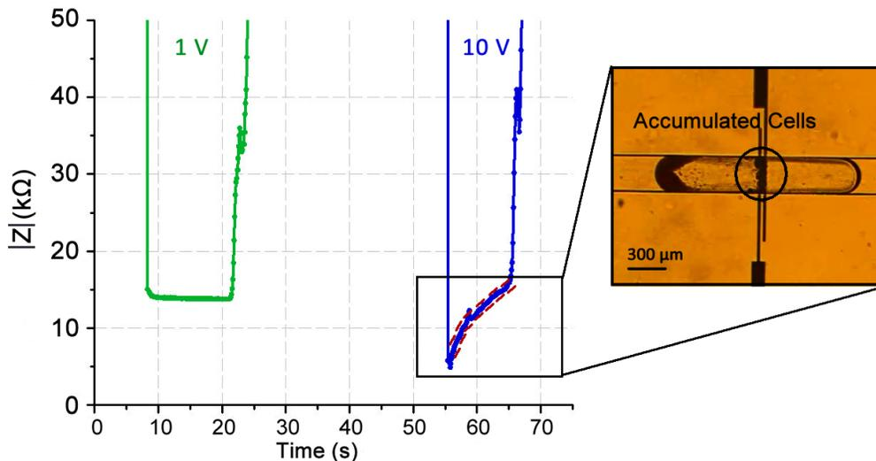
Figure 4.12: Voltage dependence of impedimetric measurement.
