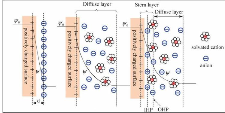
Figure 4.13: Schematic of EDL- electrical double layer on metal surface.
