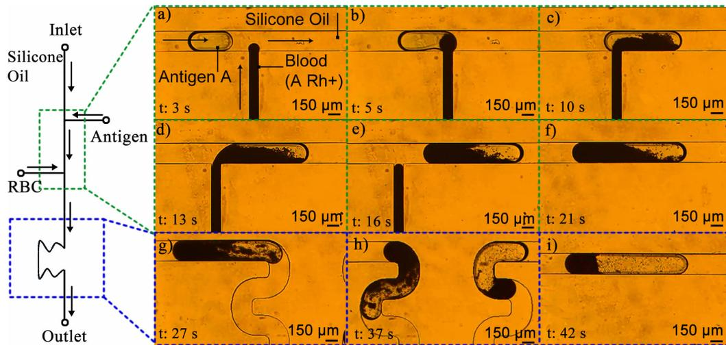
Figure 4.3: Microscope image of droplet formation.
