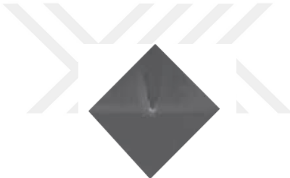
Figure 3.6 Enhanced electric-field intensity localized at a silver probe tip, calculated by the FDTD method 60
