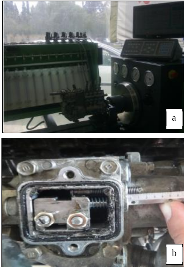
Figure 3.2.a/b. Bosch fuel-injection pump test bench / Manual readjustment of fuel pump plunger
