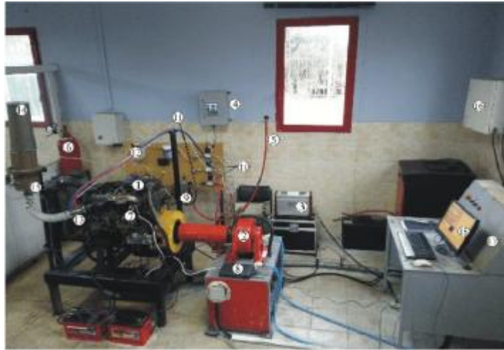
1- Engine 2- Dynamometer 3- Exhaust gas analyzer 4- Data logger 5- CNG line 6- Hydrogen tank 7- Stepping motor on fuel pump plunger 8- Stepping motor driver 9- CNG regulator 10- Flow meters 11- Needle valves 12- Gas fuels lines 13- Mixture chamber 14- Air filter 15- MAF 16- Fuel Flowmeter 17- Dynamometer Control Unit 18- Main Computer
