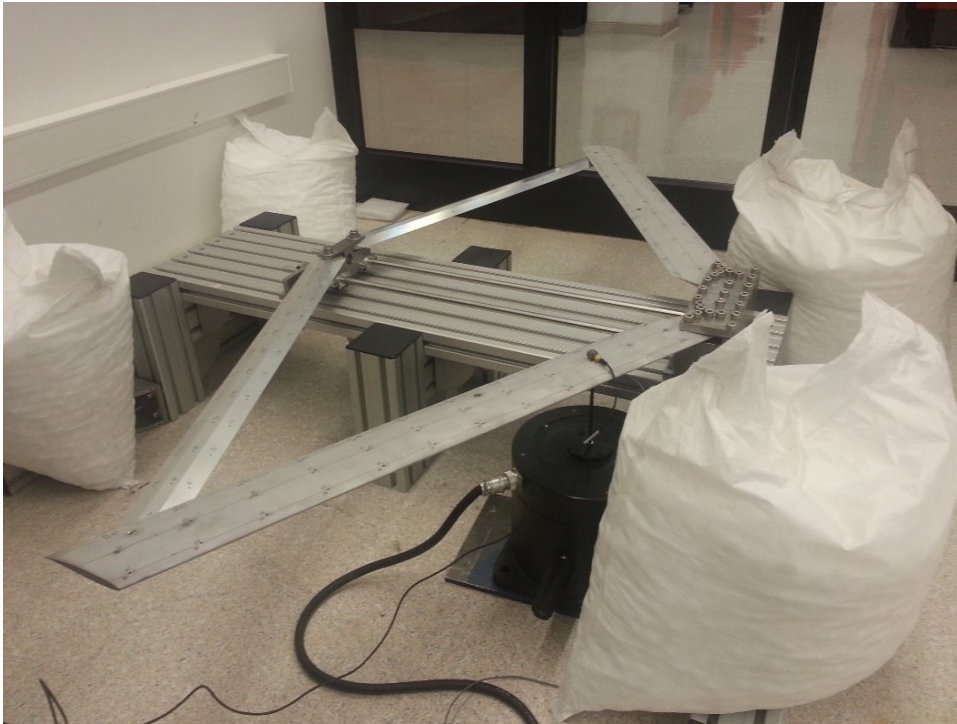
Figure 5.27. Test setup for shaker test of the Design Point 2
