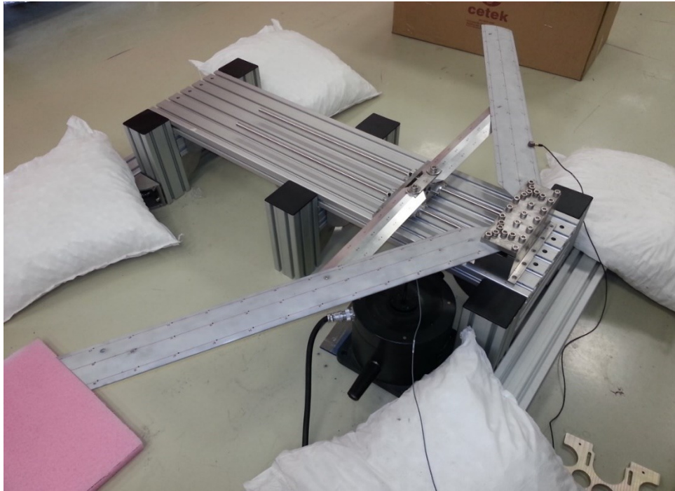
Figure 5.23. Test setup for shaker test of the Design Point 1
