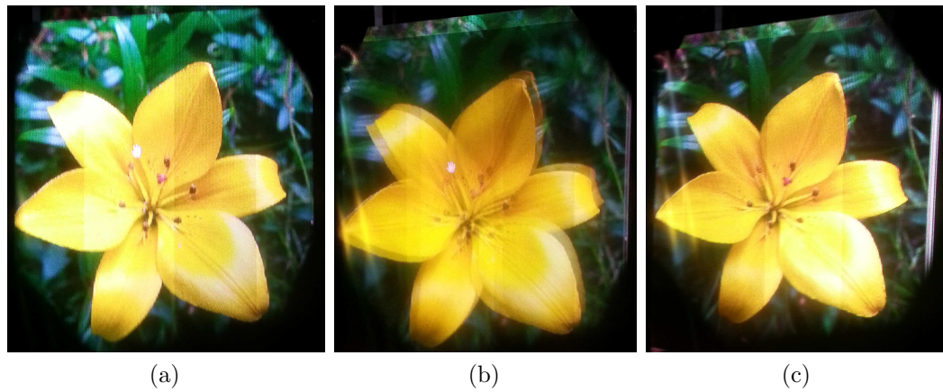
Figure 3.11: Screen shots taken from different viewing positions: (a) left eye, (b) between the two eyes, and (c) right eye.
