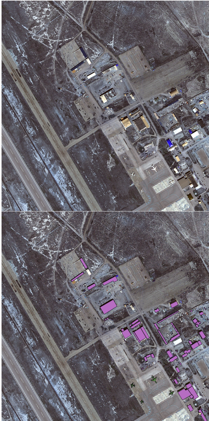
Figure 4.1: HASAT Database Example Top:Original image, Bottom:Ground truths, pinks are building, greens are aircrafts.
