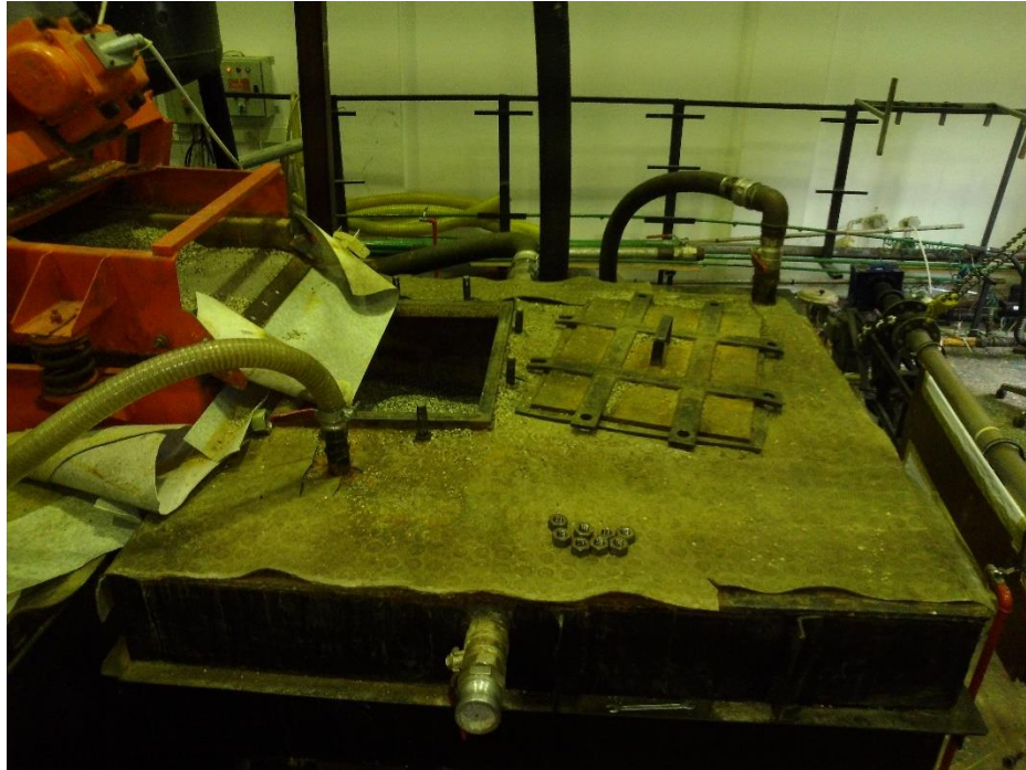
Figure 3. 8 Cuttings Collection Tank
