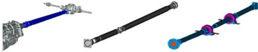
Figure 1.3: 1-piece, 2-piece and 3-piece driveshafts [1].
