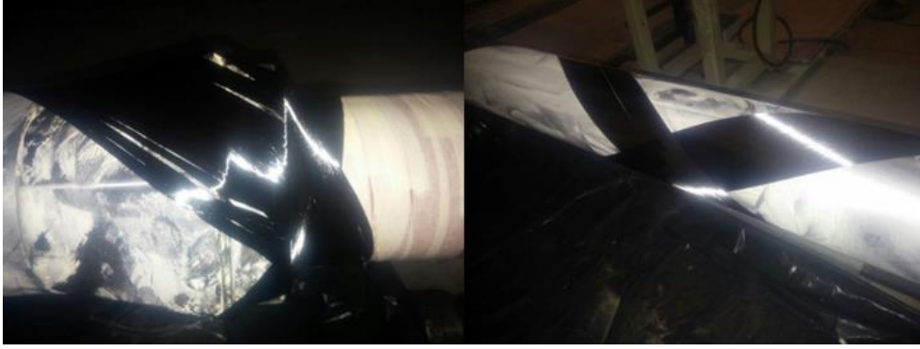
Figure 3.91: Winding with resin and masking tape.
