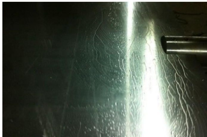
Figure 3.22: Release agent on surface of the mandrel.
