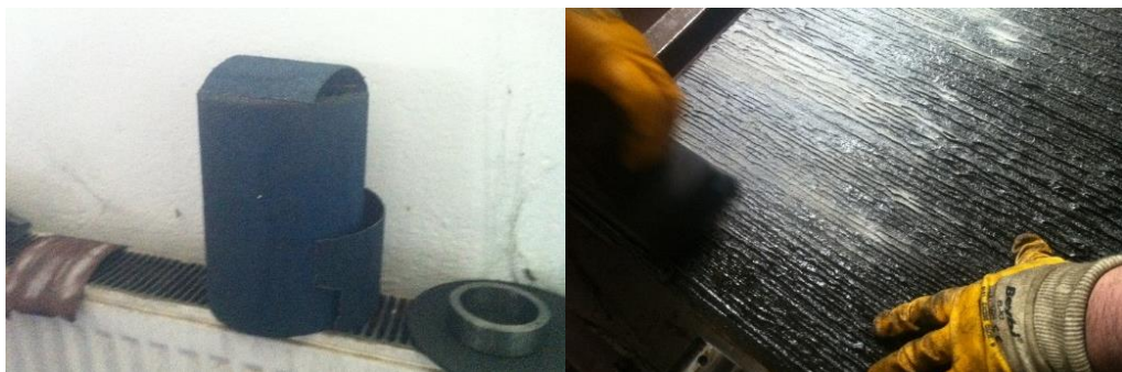
Figure 3.36: Grinding outer surfaces of the winding.
