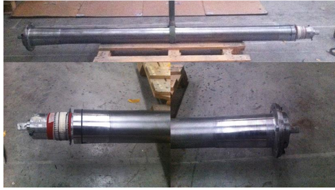
Figure 3.111: Latest configuration of mandrel and end connection parts.
