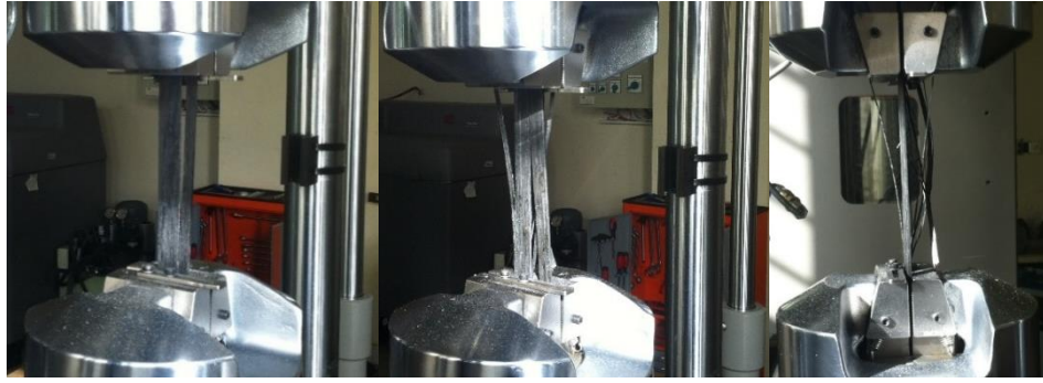
Figure 3.42: Specimens after failure on MTS322.21.
