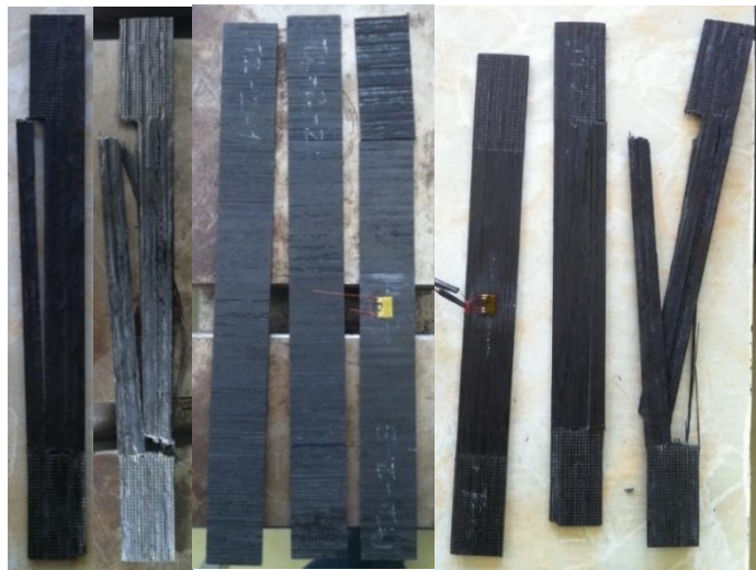
Figure 3.43: Tension specimens after failure.
