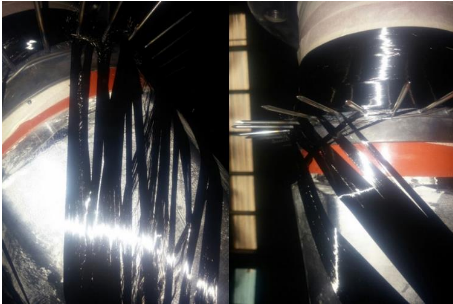
Figure 3.92: Separation of the tow between the pins.
