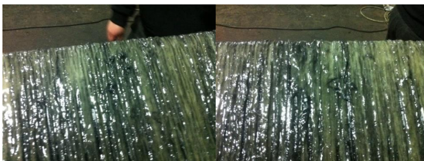
Figure 3.29: Residues stuck in the winding.
