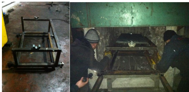
Figure 3.31: Improvised carriage for the oven.
