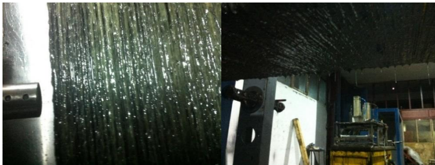
Figure 3.28: Excess resin in the winding.
