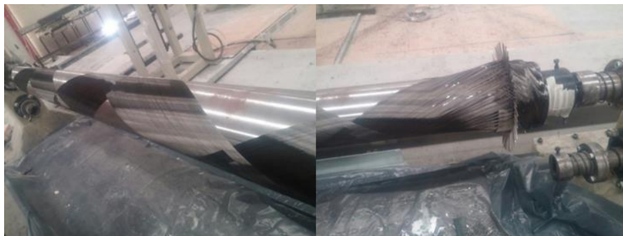
Figure 3.90: Winding with pins fixed on a ring.
