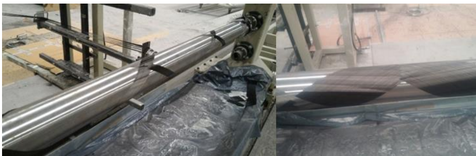
Figure 3.88: Winding on the cylindrical region of mandrel.
