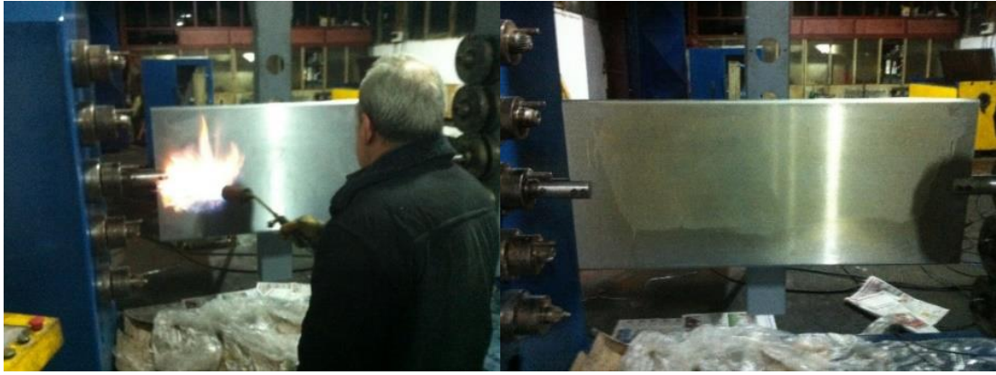
Figure 3.21: Heating of the mandrel.
