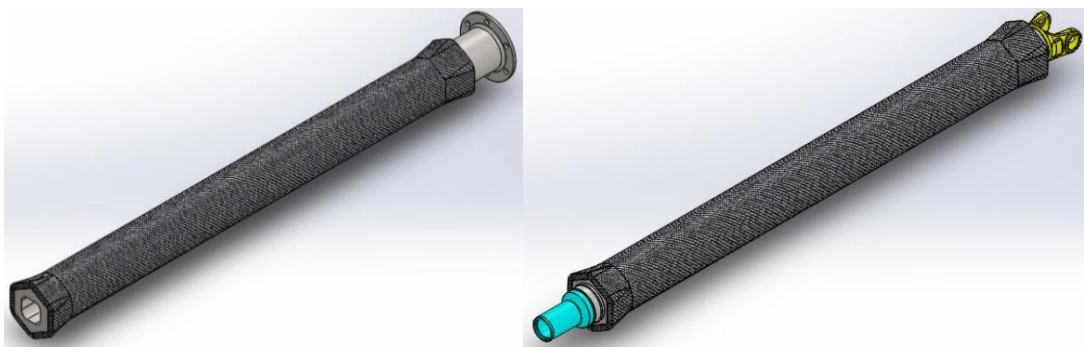
Figure 3.62: Rig and vehicle configurations of proposed driveshaft.
