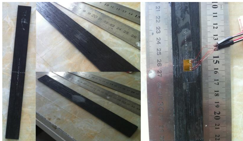
Figure 3.46: Placement of a strain gage over a specimen.
