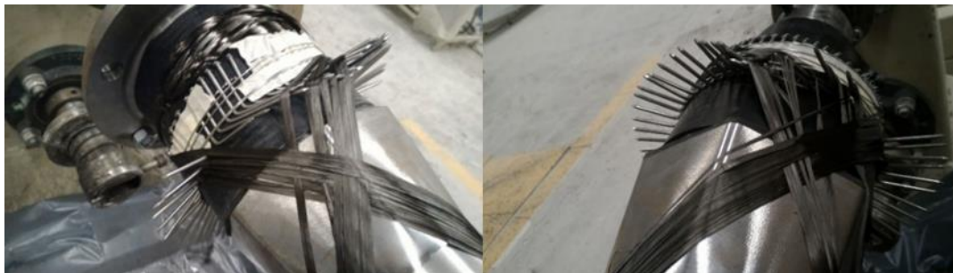
Figure 3.87: Bending of pins fixed with steel wire.
