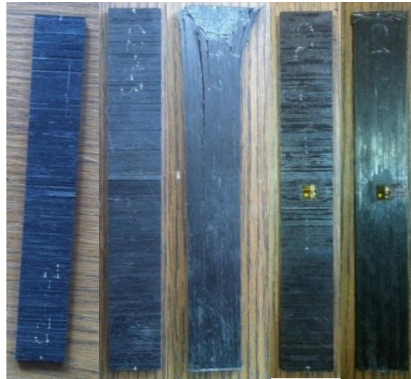
Figure 3.45: Failed compression specimens.
