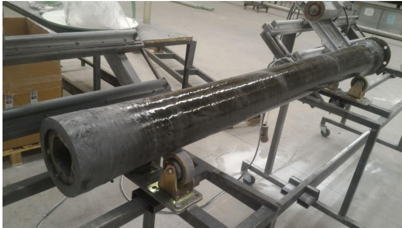
Figure 3.114: Prototype driveshaft after mandrel removal and trimming.
