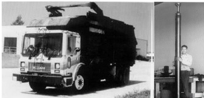
Figure 1.11: Garbage truck with composite driveshaft [2].
