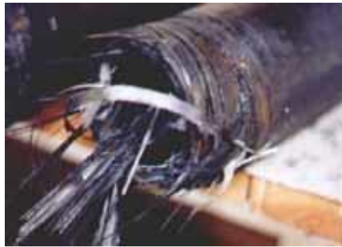
Figure 1.9: A failed composite driveshaft (Url-2 ).
