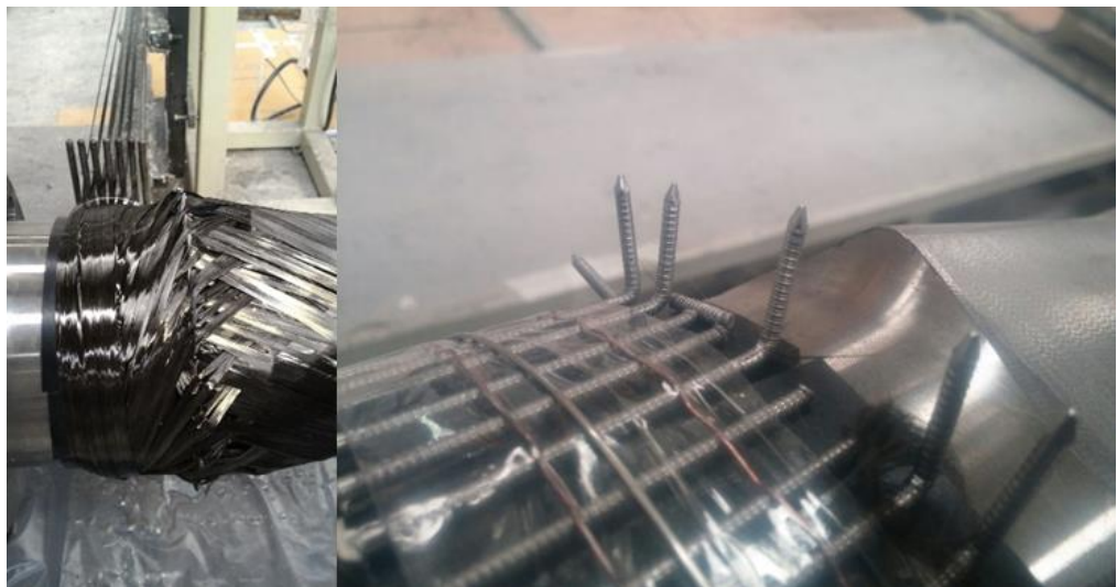
Figure 3.85: Bent and broken pins.
