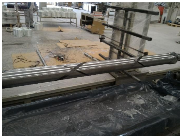
Figure 3.80: Trial winding with carbon fibers.
