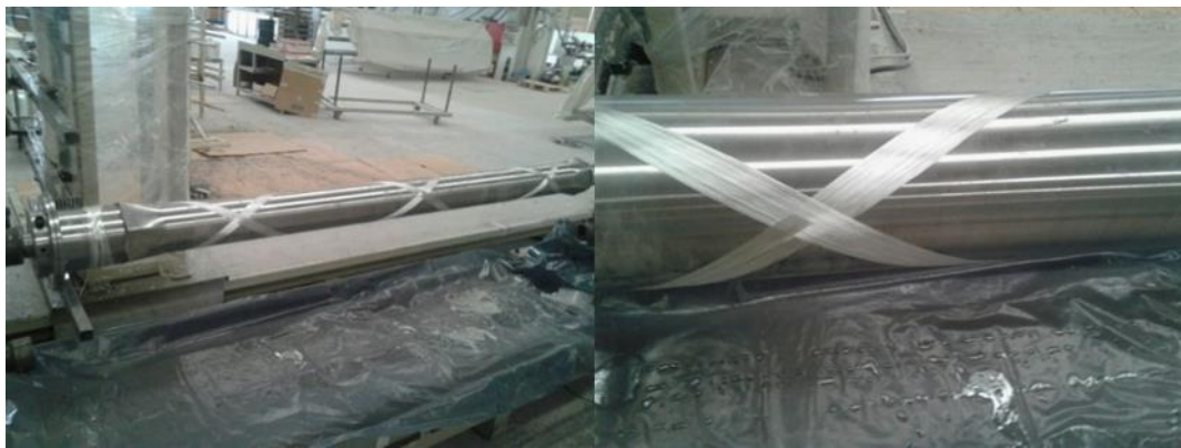
Figure 3.79: The first trial winding with glass fibers.
