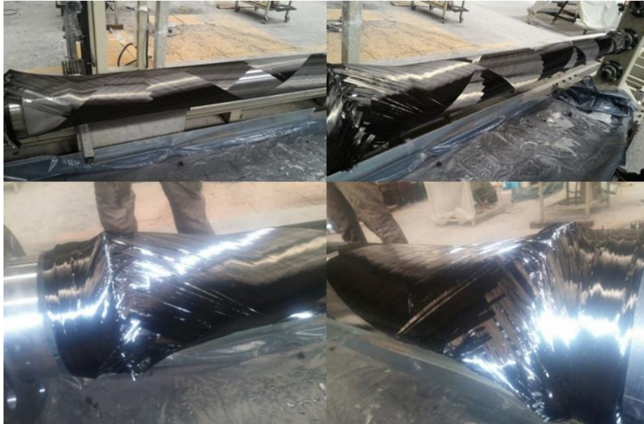
Figure 3.86: A complete layer wound for trial.
