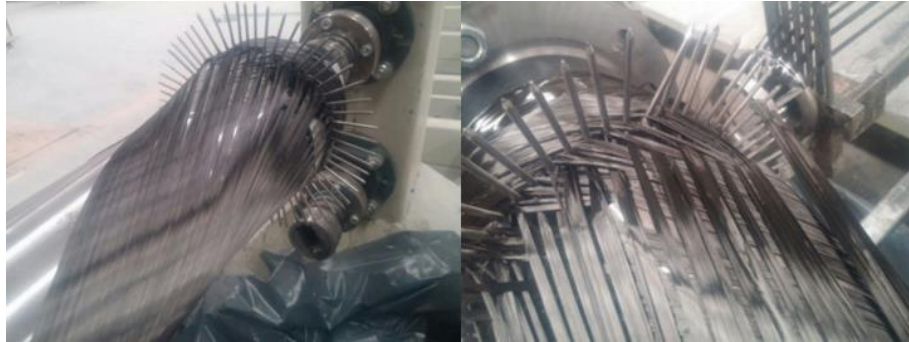
Figure 3.89: Bending of pins fixed on a ring.
