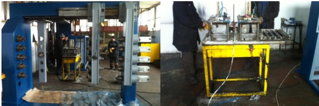
Figure 3.18: Filament-winding stand and resin bath.
