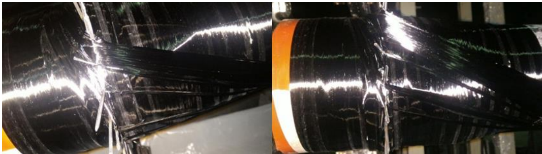
Figure 3.94: Winding on trimmed end piece.
