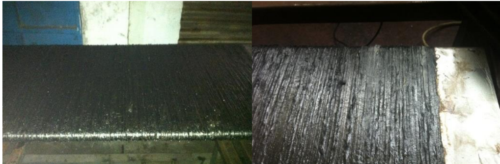
Figure 3.35: Surface roughness of the winding.
