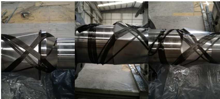
Figure 3.82: Separation of bundles over end pieces.
