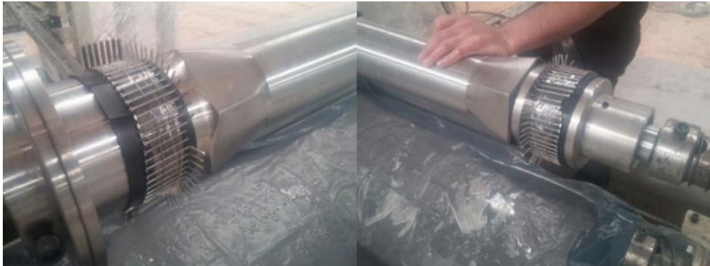
Figure 3.84: Winding pins in place.
