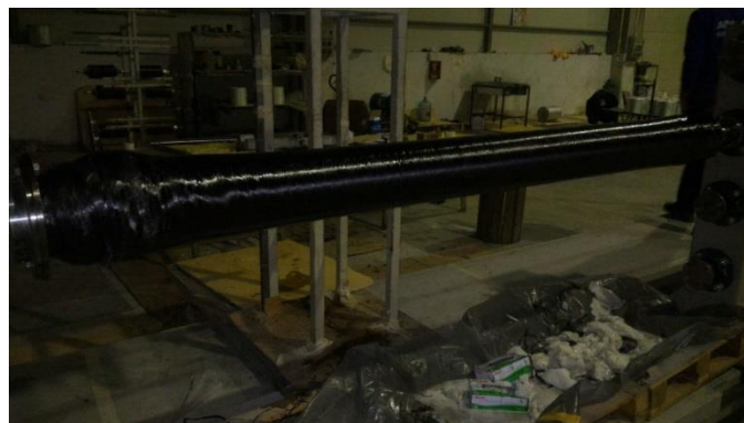
Figure 3.113: Prototype driveshaft after winding operation.
