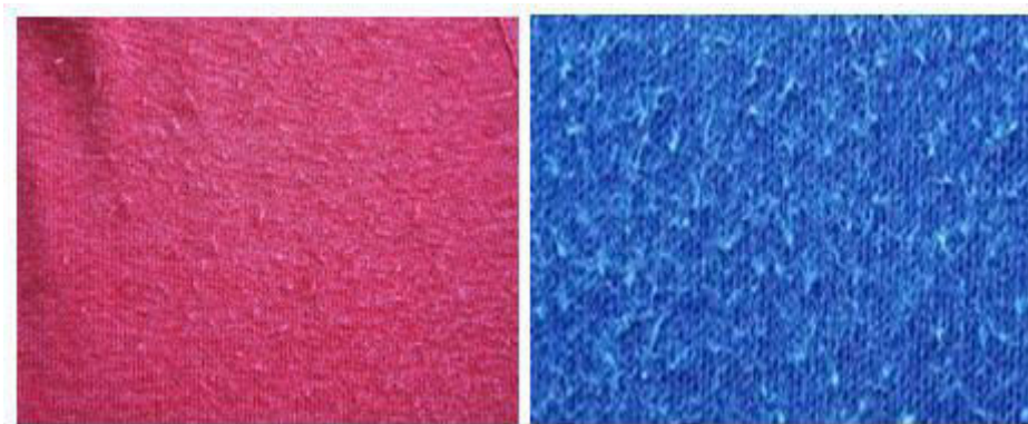
Figure 1.3 : Two different pilling examples for viscose fabric.
