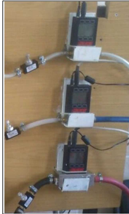
Figure 3.7. Maxtor needle vanes and Alicat flow meters.
