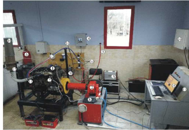
1- Engine 2- Dynamometer 3- Exhaust gas analyzer 4- Data logger 5- CNG line 6- Hydrogen tank 7- Stepping motor on fuel pump plunger 8- Stepping motor driver 9- CNG regulator 10- Flow meters 11- Needle vanes 12- Gas fuels lines 13- Mixture chamber 14- Air filter 15- MAF 16- Fuel Flowmeter 17- Dynamometer Control Unit 18- Main Computer
