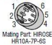
Figure 2: Hirose 6-pin Circular Male—Power Connector
