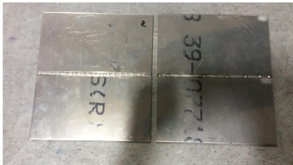
Figure 4.4 : Tack welded parts.
