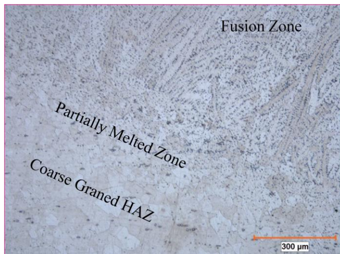
Figure 5.8 : Microstructure of weld transverse section indicatig PMZ and coarse-grained HAZ.
