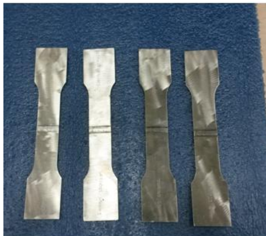
Figure 4.14 : Welded tensile specimens per ISO 4136.
