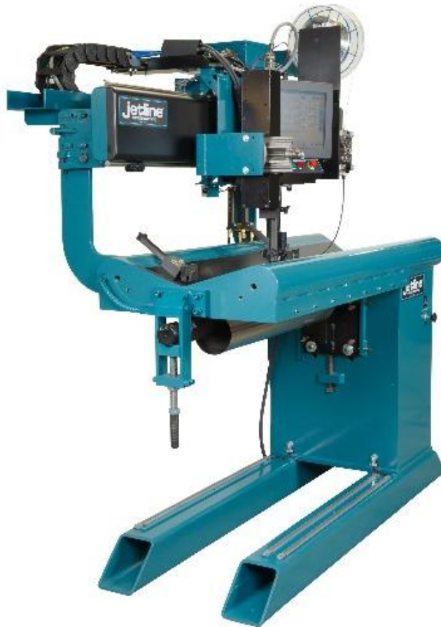
Figure 4.3 : Jetline external longitudinal seam weld machine.
