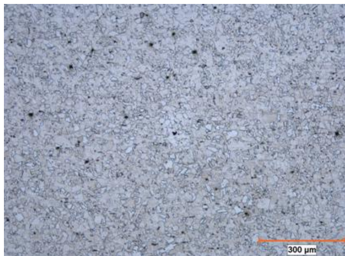
Figure 4.1 : The microstructure of as received Inconel 718 alloys (100X).
