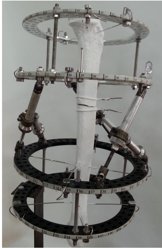
Figure 6.16. System configuration after the strut lengths are set to their final values as obtained from the GUI.
