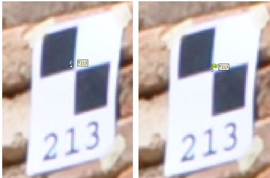
Figure 3.8 : Before and after replacing the ground control points.
