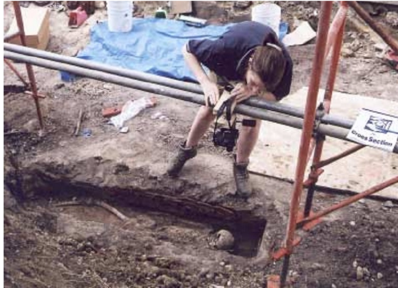
Figure 2.11 : Image capture for stereo photogrammetric techniques with the help of a scaffolding.
