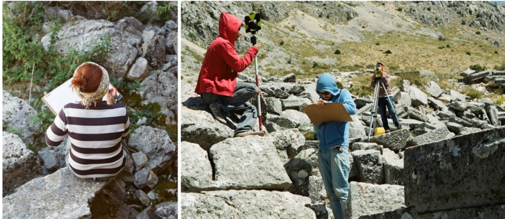
Figure 2.3 : Sketching and measuring with tacheometrical technique.
