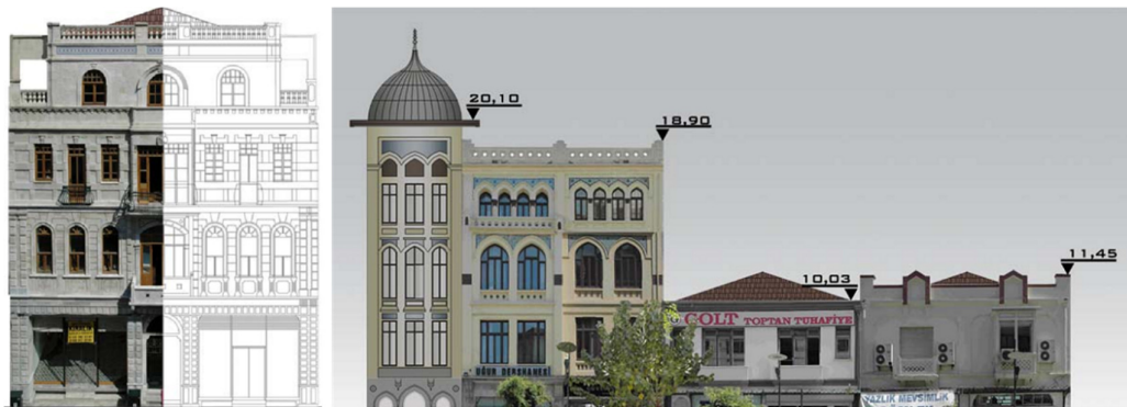
Figure 2.9 : Photogrammetric documentation of Necatibey Boulevard using rectified images.
