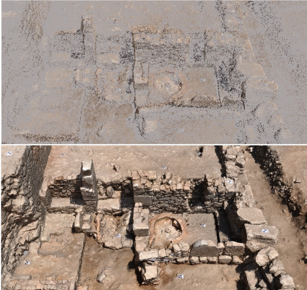
Figure 3.9 : The 3D sparse point cloud (top) created by using SfM algorithms, after the photograph alignment process, and the dense point cloud (bottom) created by using MVS algorithms, after the dense point cloud generation process.
