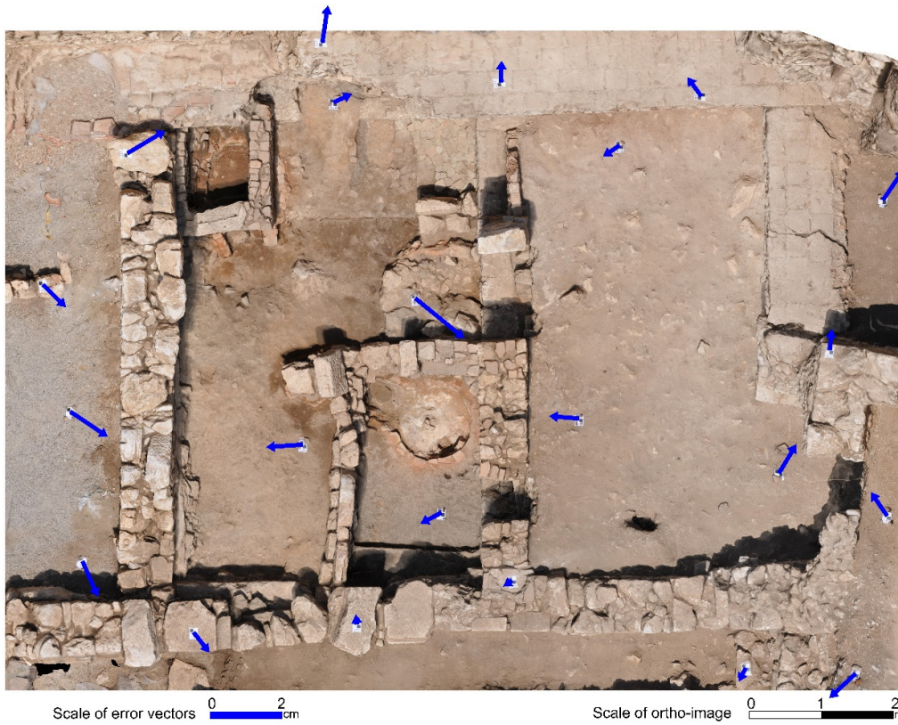
Figure 3.12 : The accuracy of the model is represented as an ortho-image including error vectors.
