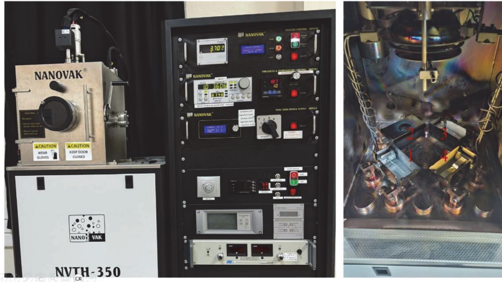
Figure 2.4. Nanovak NVTH-350 Thermal Evaporation System is shown on the left. Right image shows inside of the chamber.
