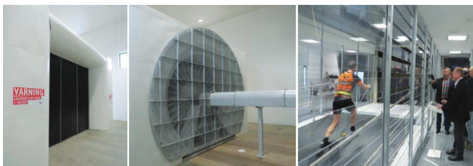
Figure 3: Wind tunnel test of ski athlete [4].
