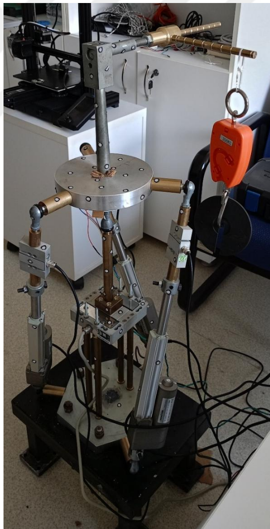
Figure 63: Measurement at (0,0,0). Force is applied on “z” axis and moment created on “x” axis.
