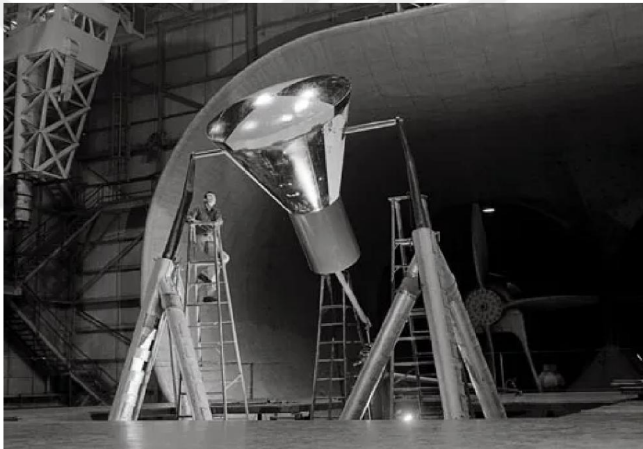
Figure 1: The Mercury re-entry capsule in wind tunnel test at NASA Langley Research Center in 1959 [1].
