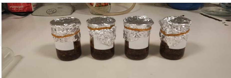
Figure 3.3 : Samples kept 24 hours without stirring during pretreatment.
