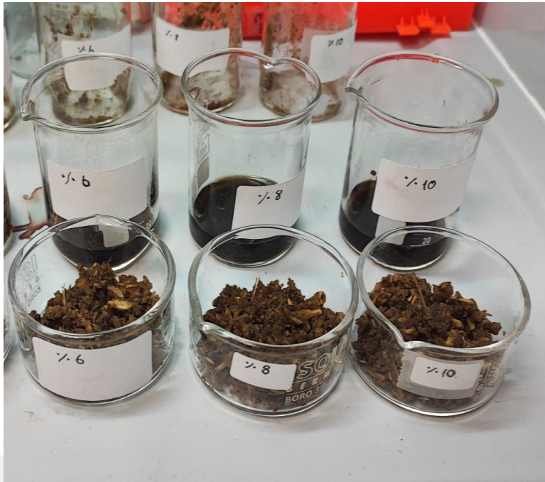
Figure 3.5 : The liquid and solid fractions after the separations of samples.
