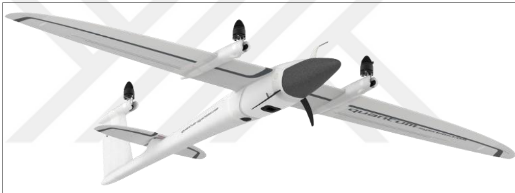
Figure 1.9: Quadplane UAV, Quantum Systems Trinity F90+ , [Web 9, 2024].
