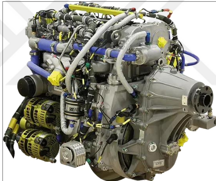
Figure 1.15: Four-Stroke Turbocharged Heavy Fuel UAV Engine , TEI PD170, [Web 15, 2024].
