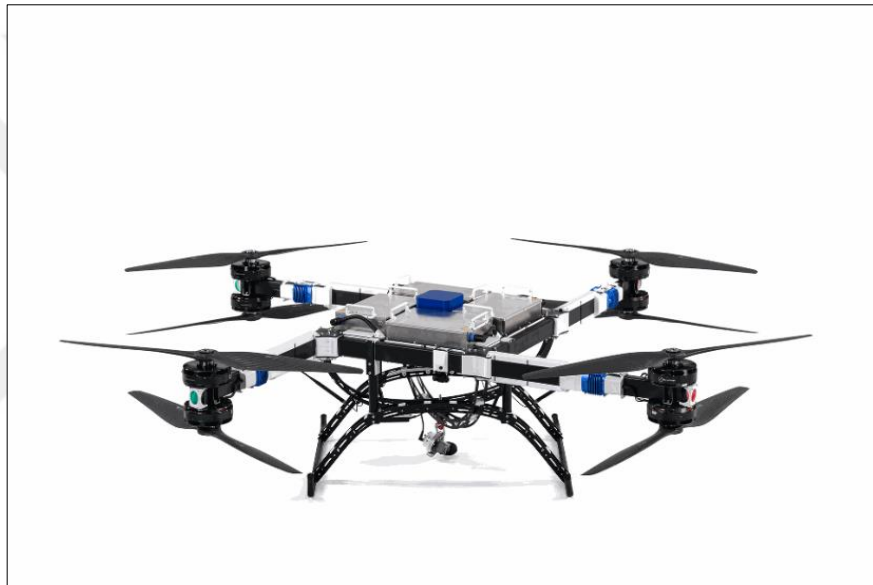
Figure 1.6: Multi Rotor UAV , FlyingBasket –FB3, [Web 6, 2024].
