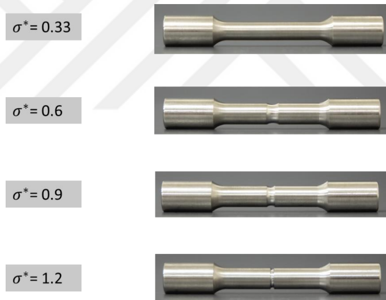
Figure 3.3. Tensile test samples with different triaxialities
