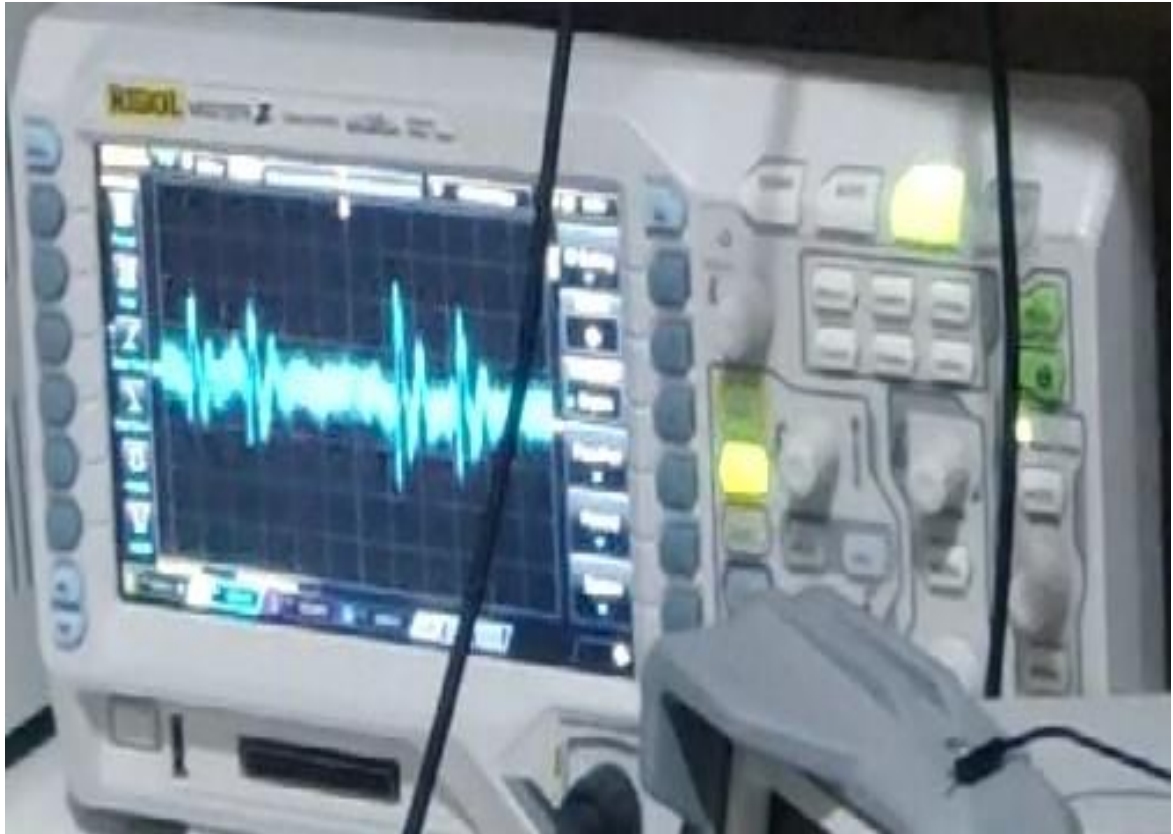
Figure 4.5. The second PCG measurement shows the distortion.
