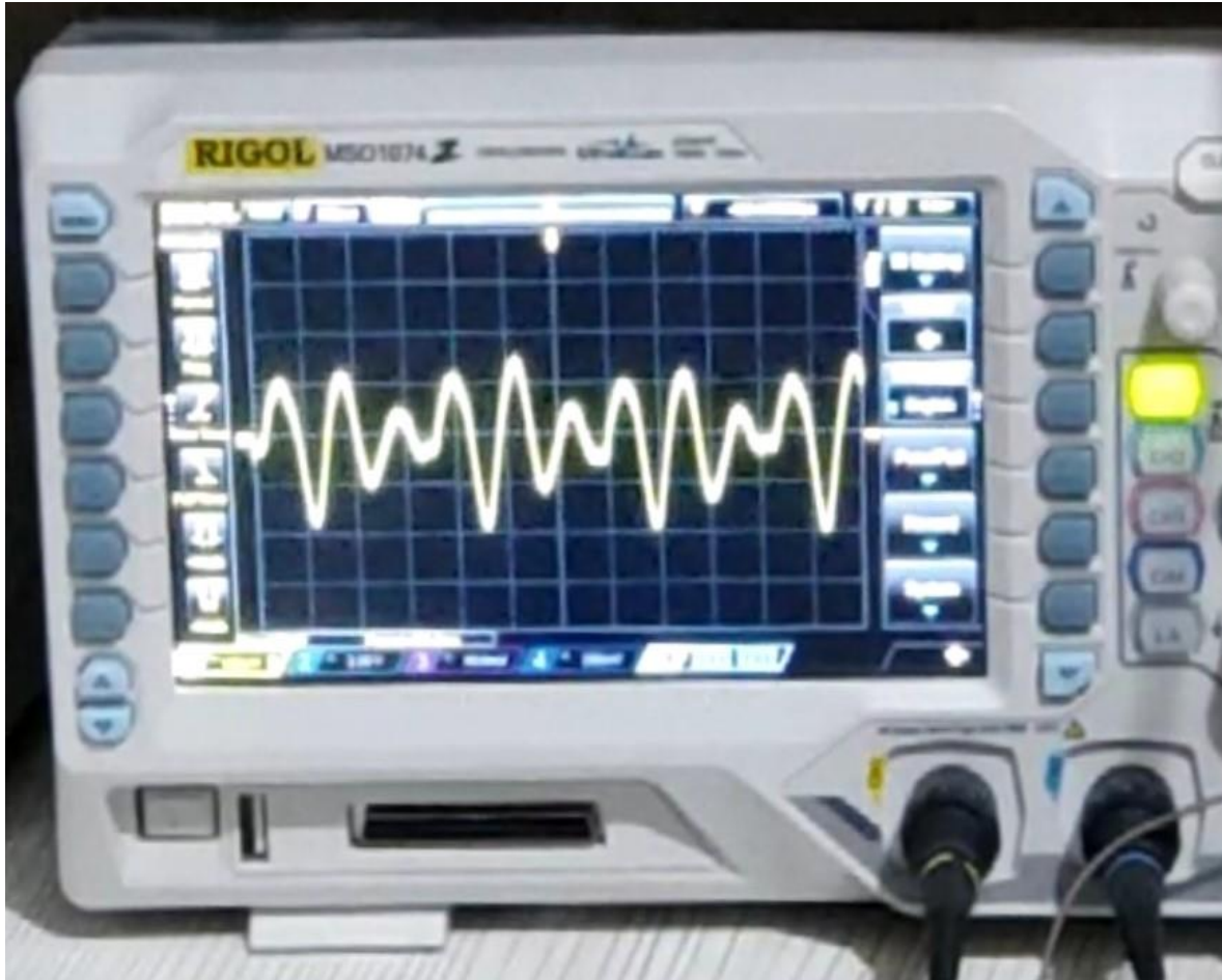
Figure 4.2. The BCG signal and its waves are shown on the screen of the oscilloscope.
