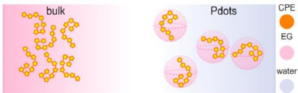
Figure 1.10. Schematic illustration of the nanophase separation method for preparation of Pdot. 29
