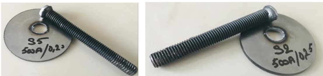
Figure 5.1 Fracture Mode on Samples After Tensile Test
