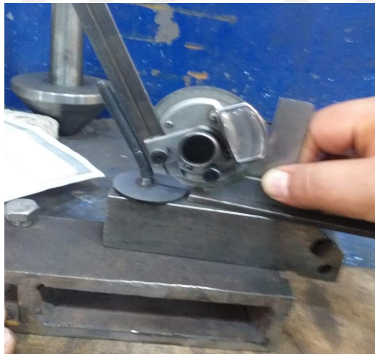
Figure 4.17 Control of Stud Bending Angle with Adjustable Mite
