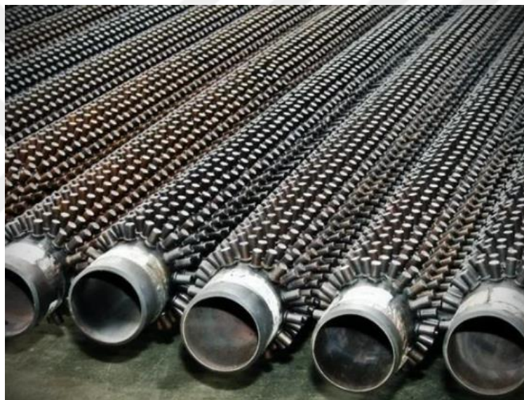
Figure 3.8 Instance of Arc Stud Welding Application in Boiler Manufacturing
