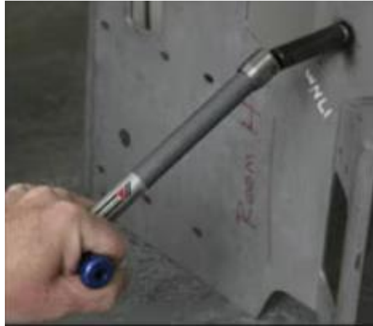
Figure 4.16 Bending Test By a Torque Wrench
