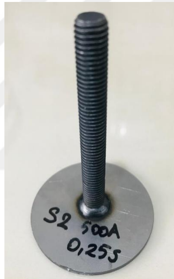
Figure 4.9 Samples Welded for Tensile and Bending Testing
