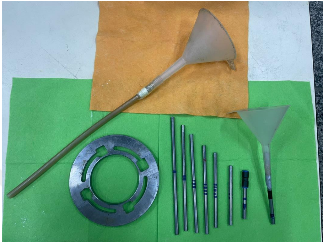
Figure 48. Air pluviation materials (centralizer, funnels, and metal pipes)
