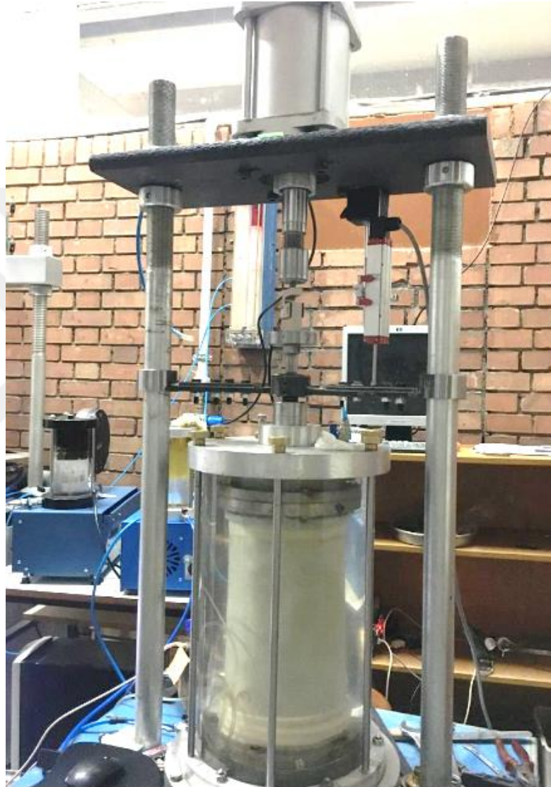
Figure 29. The hollow cylinder torsional shear apparatus used in this study
