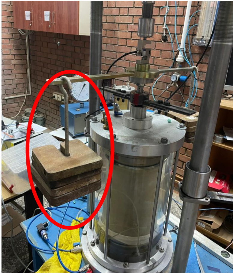
Figure 31. Dead load hangers were applied to prevent extension due to uplift
