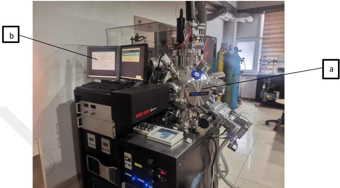
Figure 7. PED system (Neocera, Complete P180 PLD Laboratory) a) Vacuum system, b) Control System
