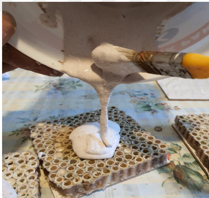
Figure 42. Pouring adhesive to bamboo core.
