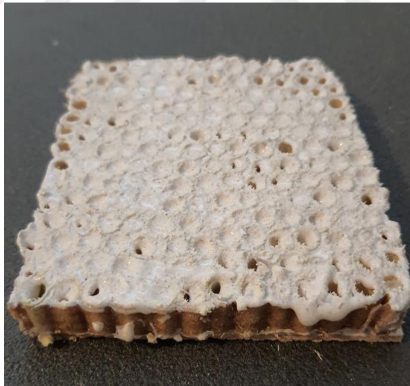
Figure 44. Bamboo core filled with d3+saw dust.
