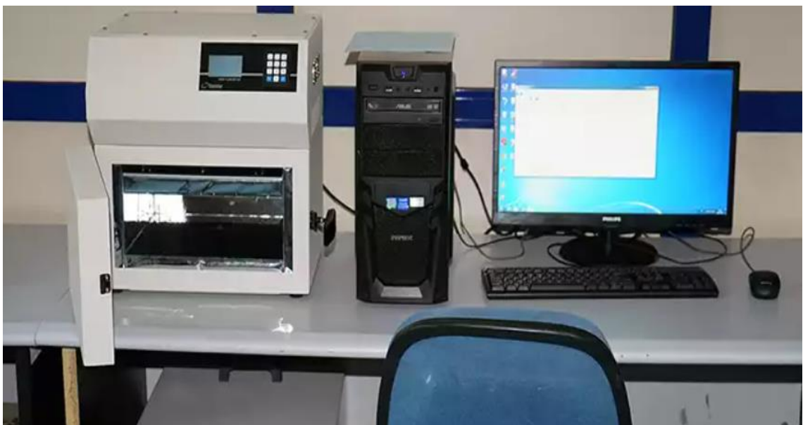
Figure 53. Thermal conductivity test machine (Brand: ThermtestHFM-100).
