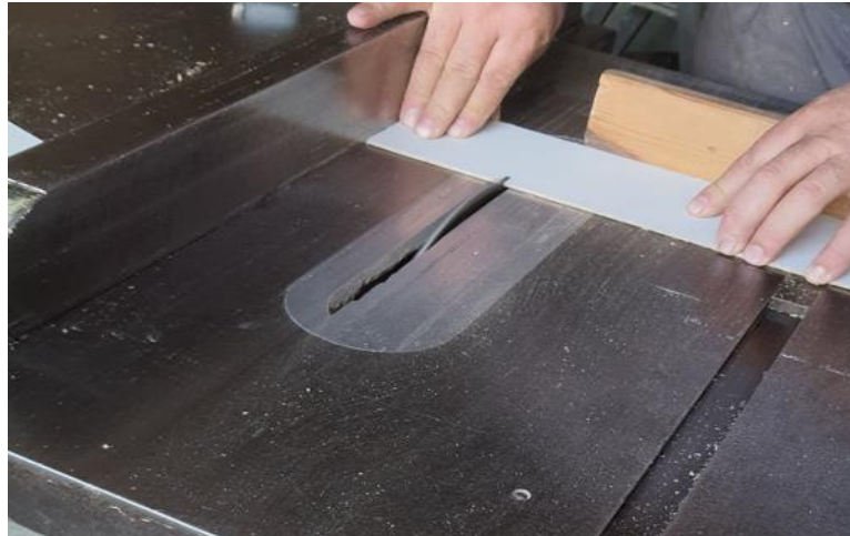
Figure 33. Hardboard 100x100 cutting with table saw machine.
