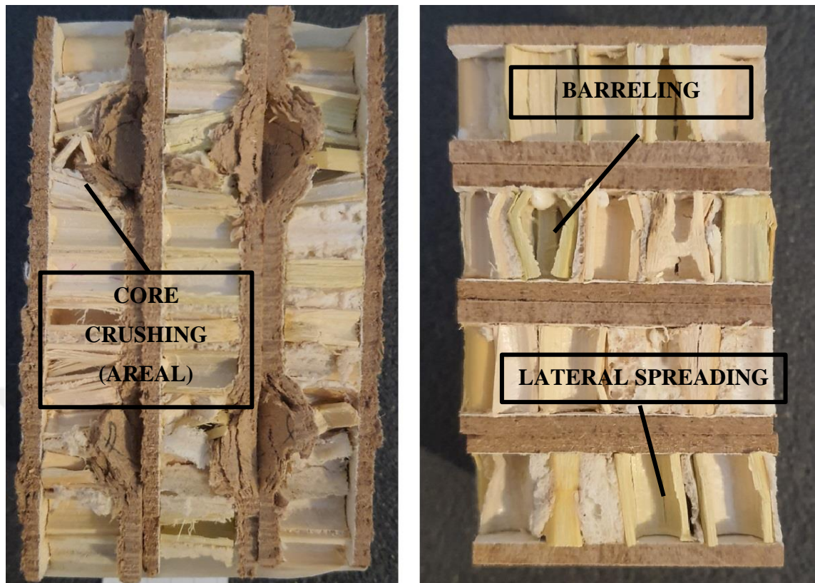
Figure 95. Side Views of Composite-4 After Indentation (left) and Compression (right) Tests.
