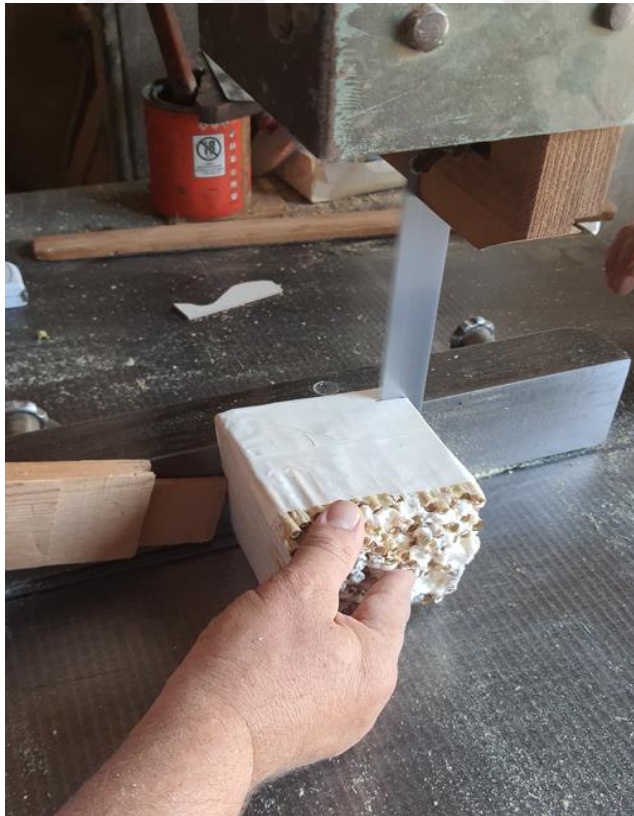
Figure 31. Material was cut by bandsaw into 12 mm thick strips.
