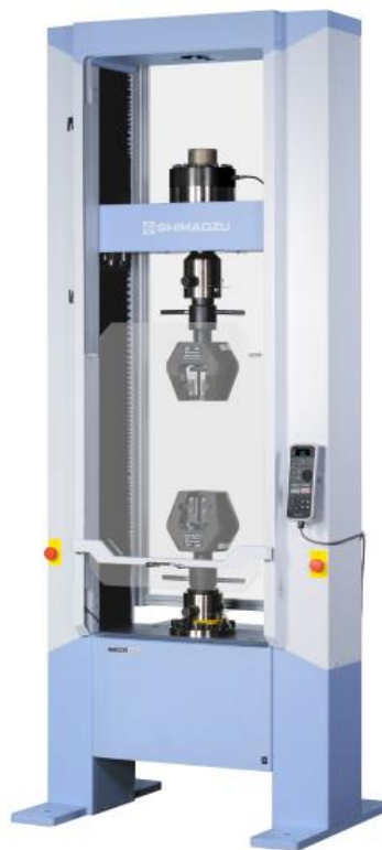
Figure 45. Compression testing machine (Brand: Shimadzu, AG-X 50kN).
