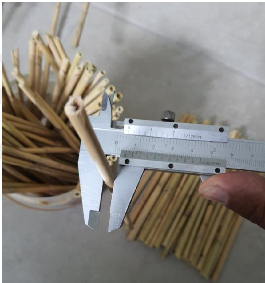
Figure 21. Measurement of bamboo diameters with caliper gauge.
