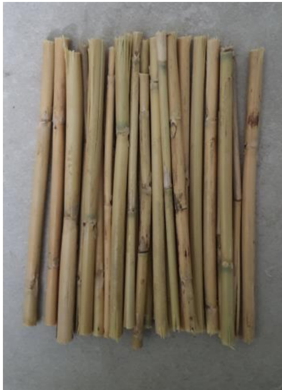
Figure 20. Bamboo cut by a band saw.
