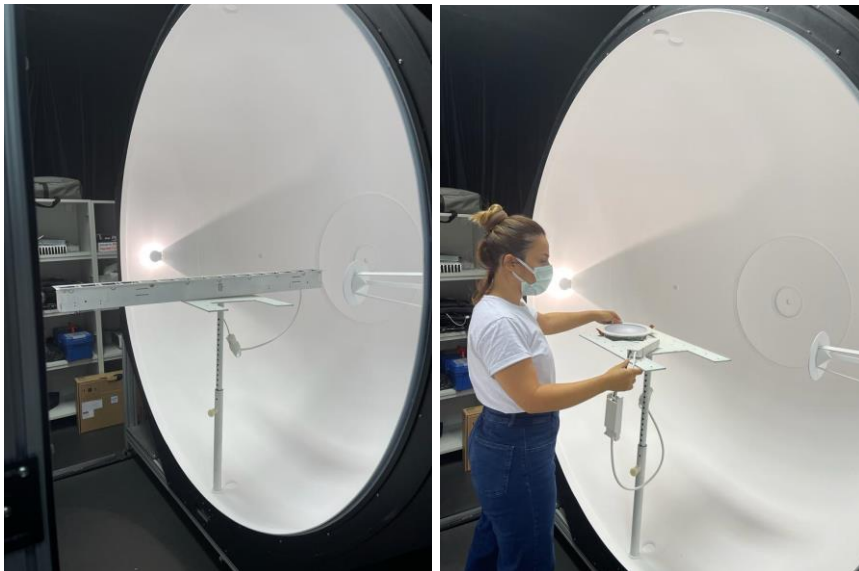
Figure 4.12: Measuring SPD of Sample luminaire.
