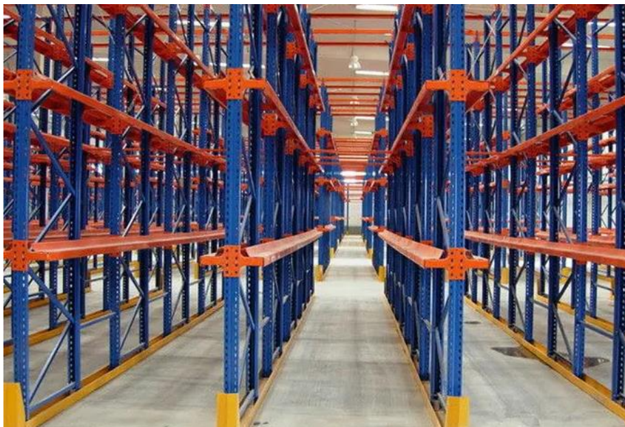
Figure 2. Drive-in drive-through rack .
