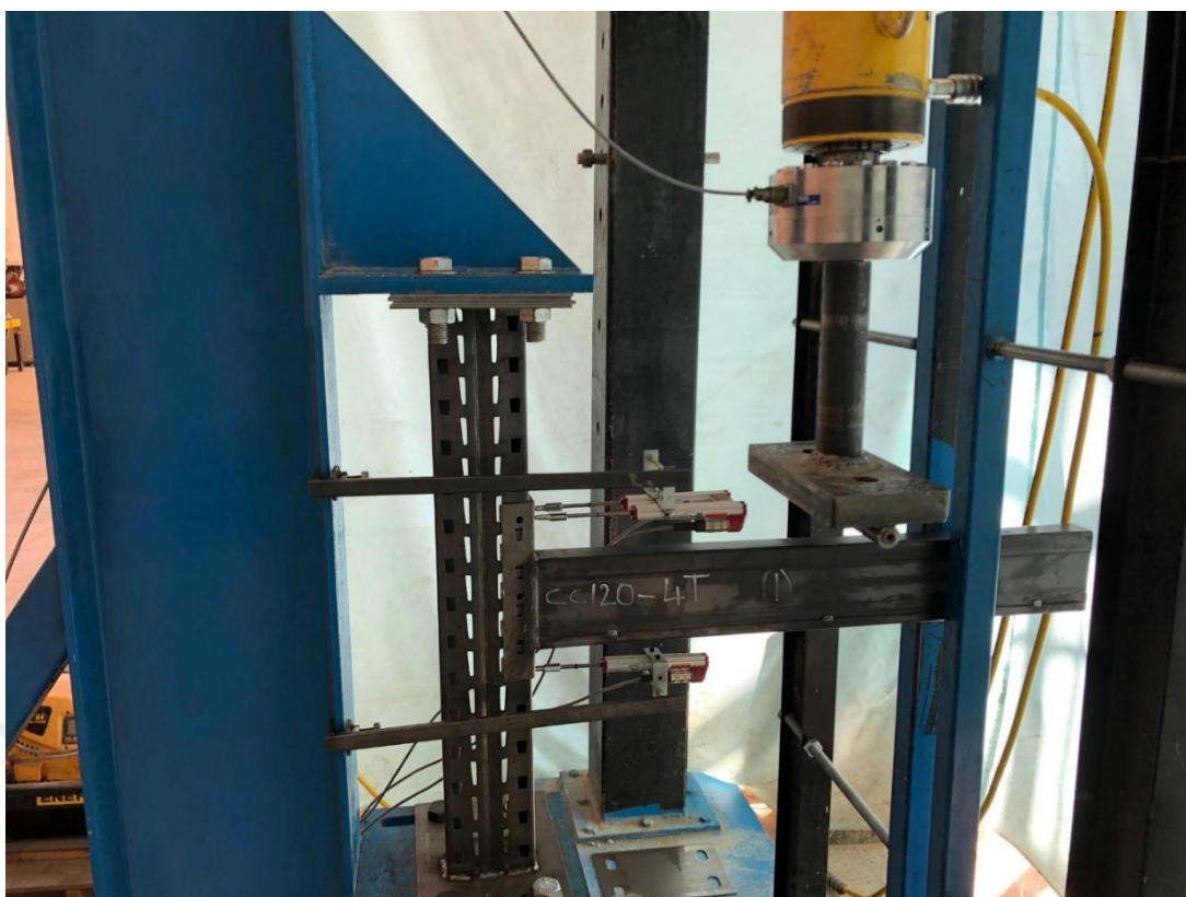
Figure 49. Single cantilever test setup.
