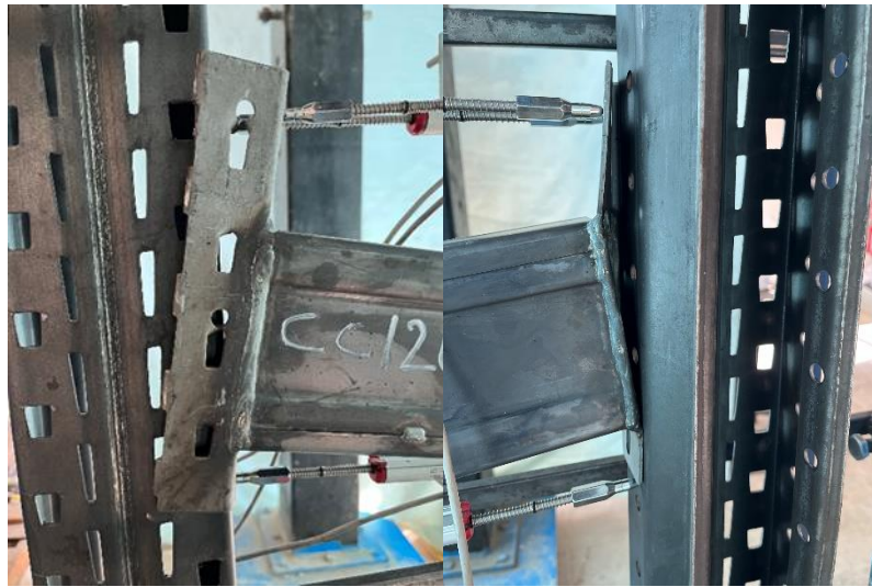
Figure 50. Failure mode A (deformation of beam end connector).
