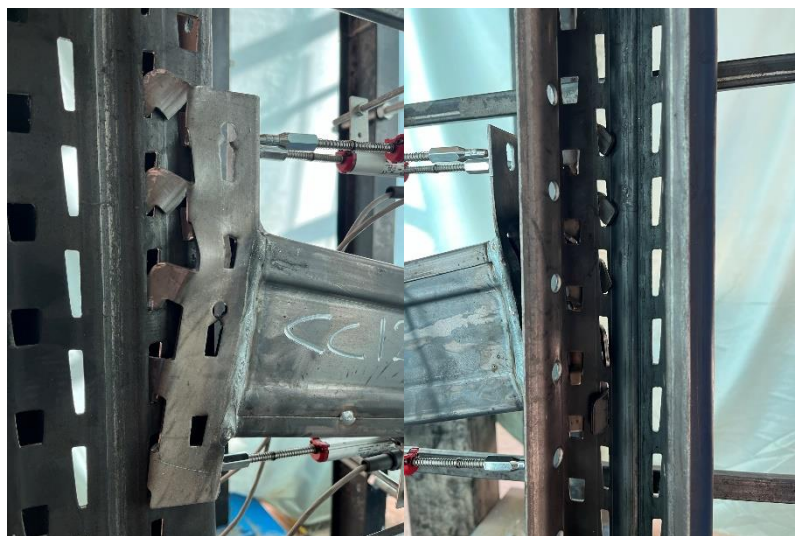
Figure 52. Failure mode A+C (deformation of beam end connector and yielding or fracture of tabs).
