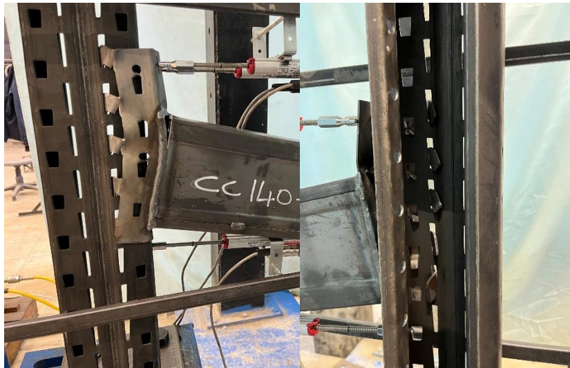
Figure 53. Failure mode A+C+D (deformation of beam end connector, yielding, and weld break).
