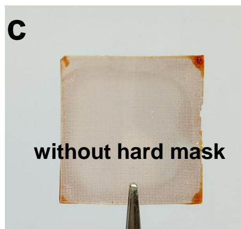
Figure 12 (a) Fourier-transform infrared spectroscopy (FTIR) analysis of three PMMA samples fabricated using different fabrication flows as Si/SiO 2 /PMMA, Si/SiO 2 /PMMA/Cu/Pr, Si/SiO 2 /PMMA/Pr, respectively, and (b-c) Optic images comparing the SU-8/PMMA substrate with and without the implementation of the hard mask technique during fabrication.
