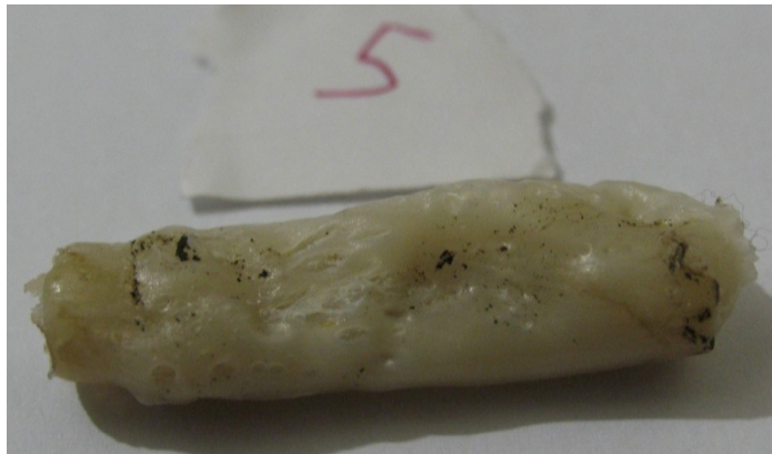
Figure IV.2 Sample 5 after MFI Test
