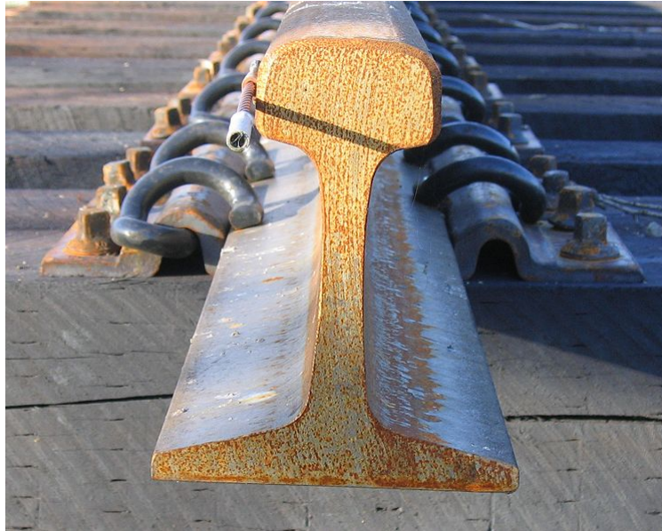
Figure 4.10: Flat bottom rail
