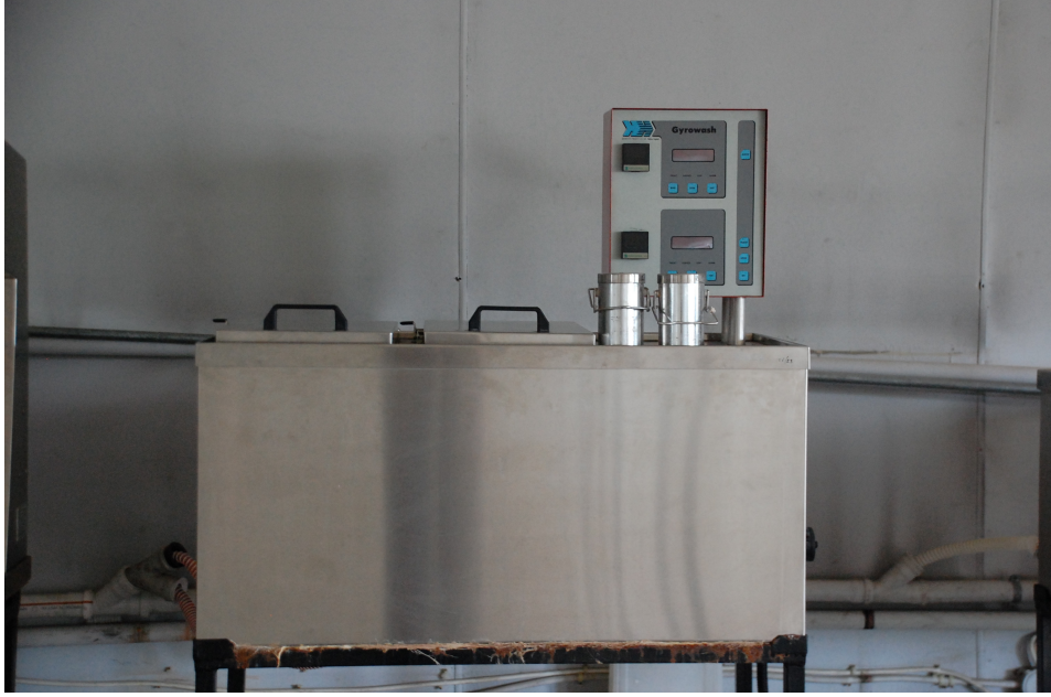
Şekil 3. 1. Gyrowash Boyama Makinesi: James H.Heal Co.Ltd. Halifax England
