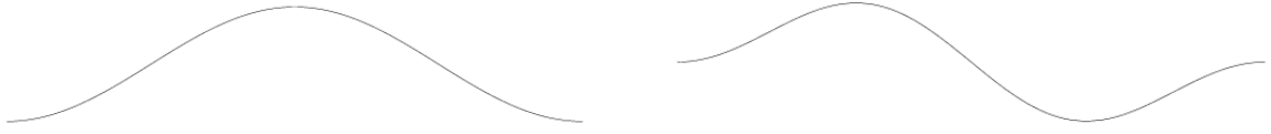
Figure 4.8. Two fixed-boundary normal modes for a beam that has attachment points at the two ends
